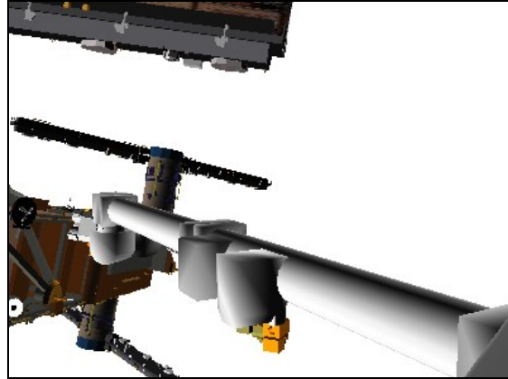
Figure 5.- Clearance 1 Position (22: Base Elbow: +145, -5).
