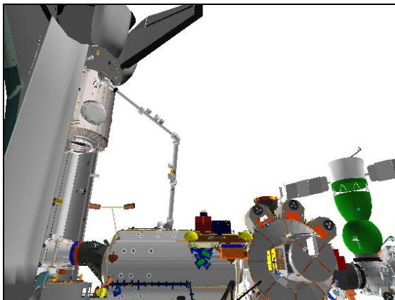
Figure 16.- Node 2 Reberth Position (03: S1 Lower Outboard: +90, +25).
