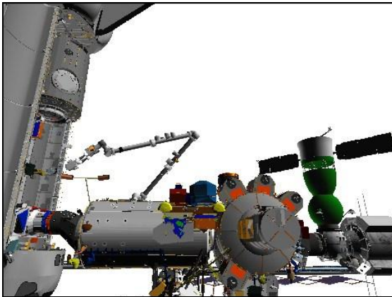
Figure 9.- PDGF Release Setup (03: S1 Lower Outboard: +95, +20).
