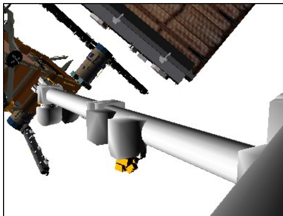
Figure 2.- P6 Ungrapple at Install (22: Base Elbow: +148, -10).
