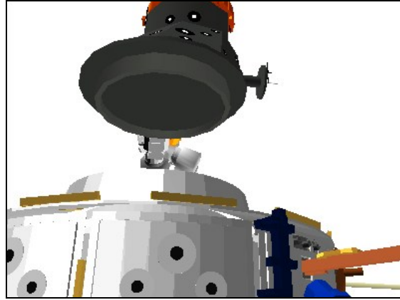
Figure 4.- PMA2 Demate (37: MBS Mast: +65, +25).
