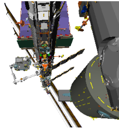
Figure 2.- ELC2 S3UO Pre-Install (SRMS Elbow: +90, -40).
