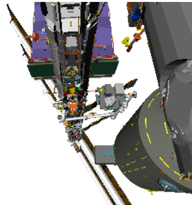
Figure 8.- ELC2 Pre-Install (SRMS Elbow: +90, -40).
