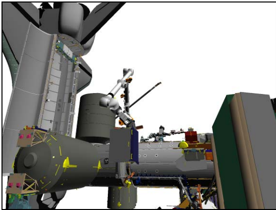
Figure 25.- ESP 2 Clearance (03: S1 Lower Outboard: +75, +20).
