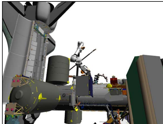
Figure 12.- ESP-2 Clearance (03: S1 Lower Outboard: +75, +20).
