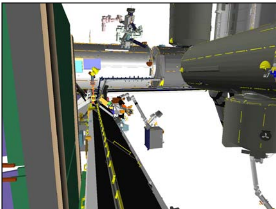
Figure 49.- Truss Clearance (09: P1 Lower Outboard: +105, -10).
