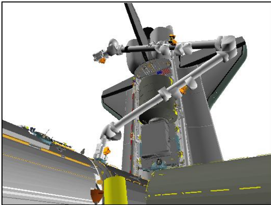
Figure 1.- Docking Park Position (07: P1 Lower Inboard: +150, +35).
