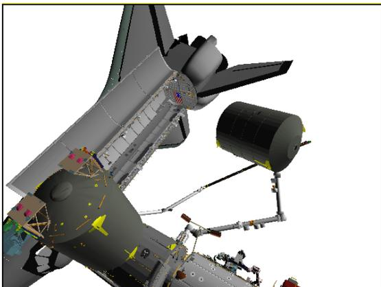
Figure 13.- PMM Intermediate 2 Position (03: S1 Lower Outboard: +100, +65).
