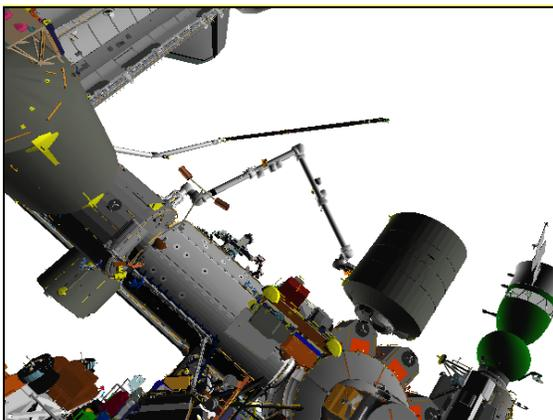
Figure 3.- PMM Node 1 Pre-Install Position (03: S1 Lower Outboard: +120, +45).
