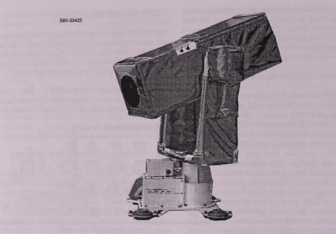
Pan/Tilt Unit with Camera Thermal Blankets
