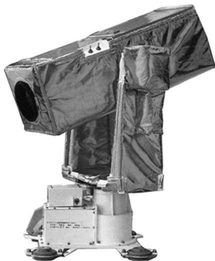
Pan/Tilt Unit and Camera with Thermal Blankets
