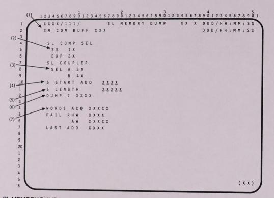
SL MEMORY DUMP is a specialist function (SPEC 111) available in PL OPS 9. This display provides control and monitoring for Spacelab Subsystem (SS) or Experiment (EXP) Computer memory dump during prelaunch checkout.
