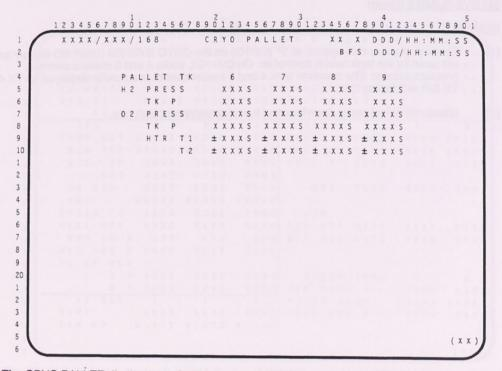
The CRYO PALLET display is an SM display (DISP 168), available in BFS SM OPS 0, which provides the crew summary level data on the EDO cryo pallet.
