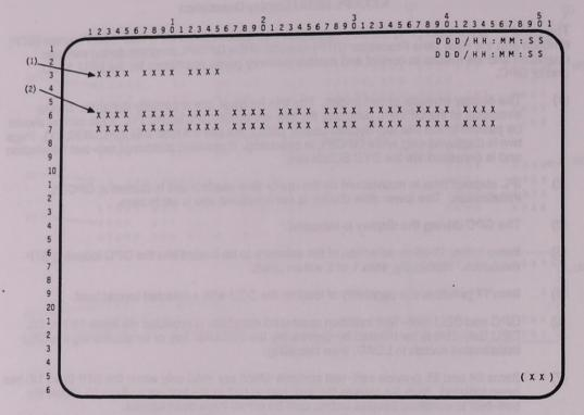
The Operational Test Program (OTP) provides the capability to test/troubleshoot the Display Electronic Unit (DEU) hardware and software. The testing does not require a GPC interface with the DEU and is available whenever the DEU Control Program (DCP) is in control (i.e., anytime after a successful DEU IPL).
