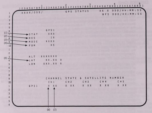
GPS STATUS is available in BFS GNC OPS 1, 3, and 6. It provides insight into GPS systems operation and health, as well as GPS-estimated position. These data are for evaluation purposes only; they are not currently used for vehicle GNC.
