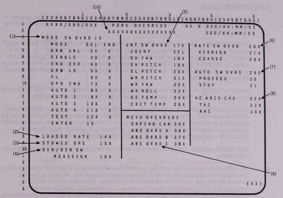
The PDRS OVERRIDE display is a specialist function (SPEC 95) available in SM OPS 2 and 4 which provides the following capabilities: override a number of RMS switch inputs in the event a major switch fails; toggle the loaded rate limit flag; and configure the RMS software for correct operation in the MPM stowed position.
