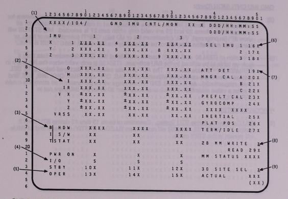
GND IMU CNTL/MON is a specialist function (SPEC 104) available in GNC OPS 9. This display supports IMU ground calibration, attitude determination, platform positioning, gyrocompassing, inertial, and TERM/IDLE functions. In addition, this display provides for a Mass Memory Read or Write of calibration parameters.
