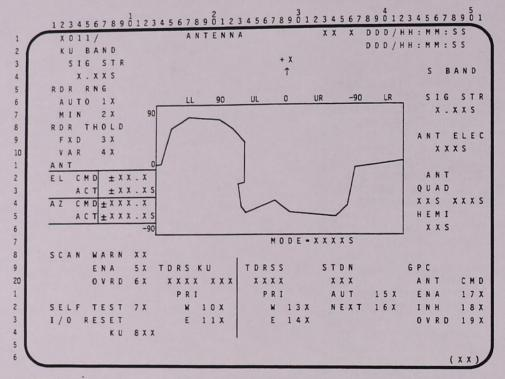
The ANTENNA display is an operations sequence (OPS X011) available in SM OPS 2 and 4 which allows control of GPC sequences for the S-band and Ku-band antenna systems.
