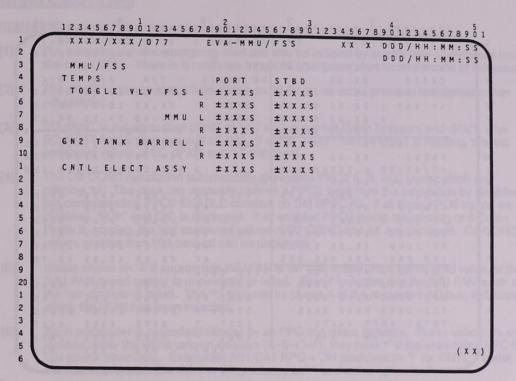
The EVA-MMU/FSS display is an SM display (DISP 77) available in SM OPS 2 and 4. It is used for thermal monitoring of the Manned Maneuvering Unit (MMU) and its associated Flight Support Station (FSS) prior to operational use and during reservicing of the GN2 propulsion system. The crew may also view the display as a result of an FDA alert/CRT message.
