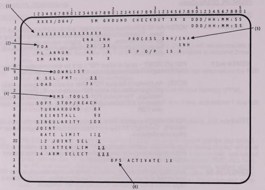
The SM GROUND CHECKOUT display is a Systems Management (SM) specialist function (SPEC 64) available in SM OPS 2 and 4 which allows the ground checkout user to modify certain SM processes to enhance vehicle turnaround and test processing. All inputs to this spec are rejected when the SM ground checkout discrete is disabled (item 52 on the DPS UTILITY display with no '\*').
