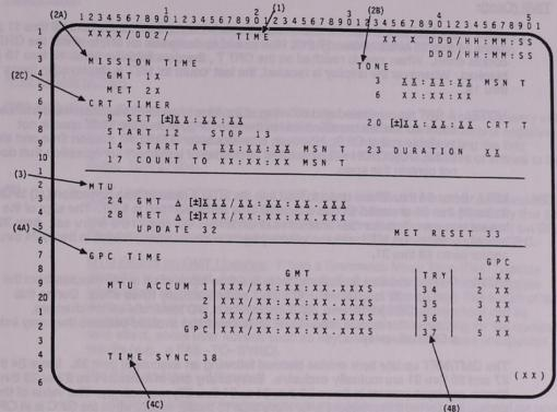
TIME display. A system level specialist function (SPEC 2) available in all OPS sequences except GNC OPS 1, 3, and 6. Includes: (2A) controls for MISSION TIME (MT) and the (2C) CRT TIMER (CRT T) for all CRT displays; (3) controls to update the Master Timing Unit (MTU – both Greenwich Mean Time (GMT) and Mission Elapsed Time (MET)); and (4A) controls to monitor and manage the GPC TIME sources.
