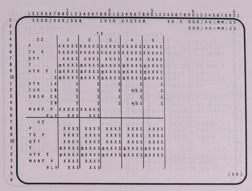
The CRYO SYSTEM display is an SM display (DISP 68), available in SM OPS 2 and 4 which provides detailed status information on the cryogenic (CRYO) subsystems.
