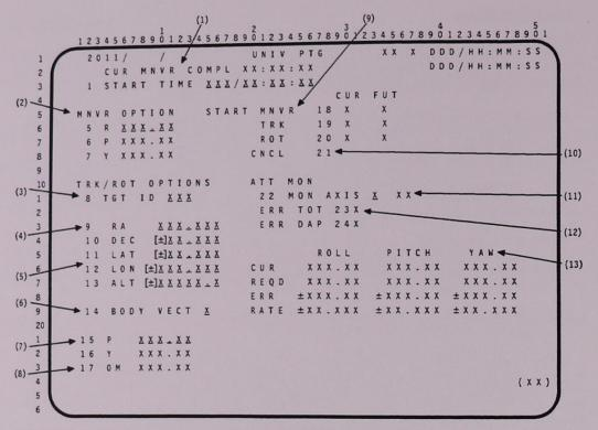
UNIV PTG. A GNC OPS display available in OPS 2 (OPS 2011). This display provides data and controls for auto attitude options and monitoring attitudes, errors, and rates. See table for units and limits.
