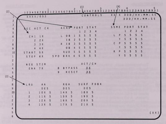
(1) CONTROLS is a specialist function (SPEC 53) available in GNC OPS 1, 3, and 6. This display provides the capability to control secondary actuator checks and deselection/ reselection of AAs, RGAs, and aerosurface position feedback transducer strings. This display also allows the crew to monitor the status of the aerosurface and SSME actuator secondary ports.
