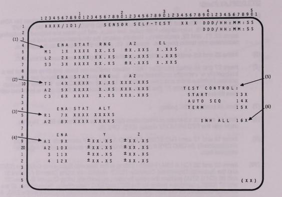
SENSOR SELF-TEST is a specialist function (SPEC 101) which is available in GNC OPS 9. This display provides the means to enable self-testing of the Microwave Scan Beam Landing System (MSBLS), the Tactical Air Navigation (TACAN), the Radar Altimeters (RA), and Accelerometer Assemblies (AA).
