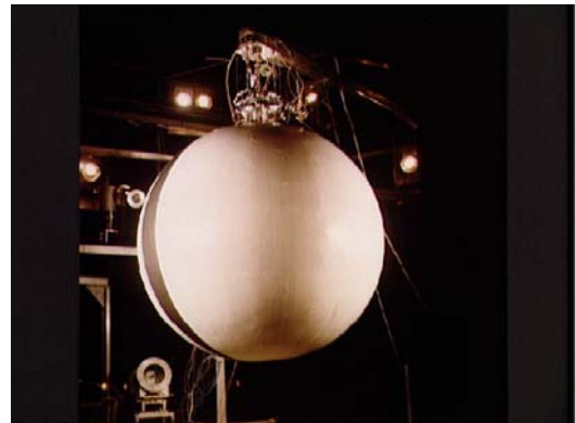
Figure 3 Test inflation of the back-up IRT balloon in a thermal vacuum test chamber.
