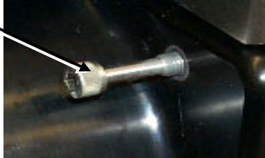
Figure 6.- Bolt Removed Too Far (Should See Only One Thread).
