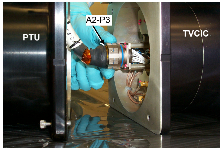
Figure 4.- Connection from Pan Tilt Unit to TVCIC.
