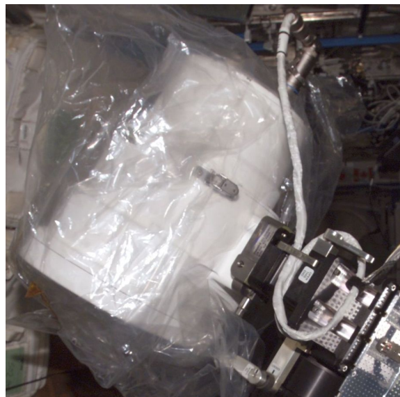
Figure 8.- ETVCG Light Installed on ETVCG With Protective Packaging Left in Place.
