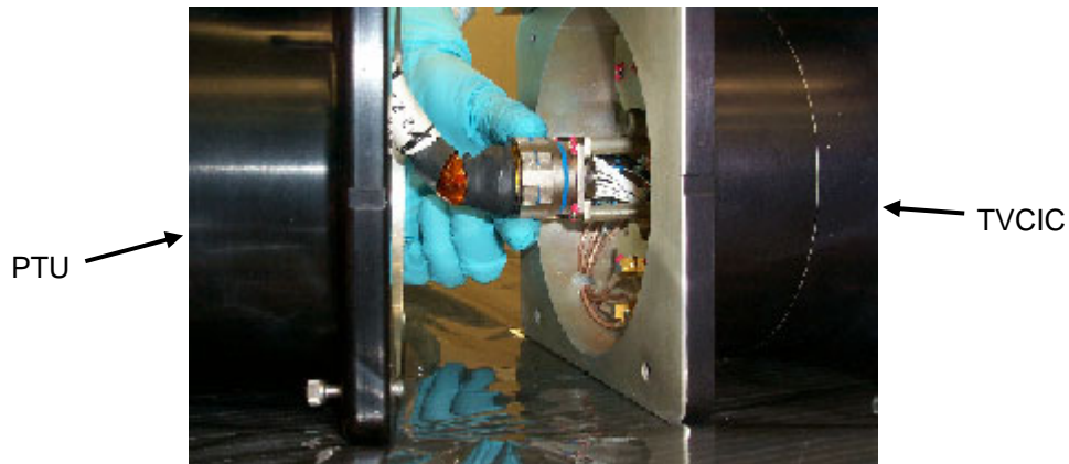
Figure 4.- Connection from Pan Tilt Unit to TVCIC.
