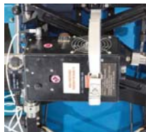
⑦ Restrain ICU and seat legs using extension strap
