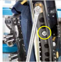
② Install bushing into port side of seat back
