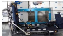
⑨ Open seat pan(s) into entry config (pull gold T-handles on port & stbd seat back to release seat pan(s))
