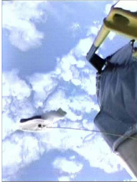
Figure 1. Grounding Tab Obstructing Camera View
