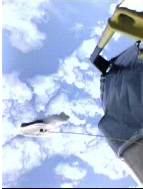
Figure 1. Grounding Tab Obstructing Camera View
