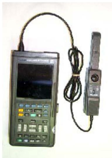
Figure 4. Scopemeter Current Probe Connected to Scopemeter INPUT A.
