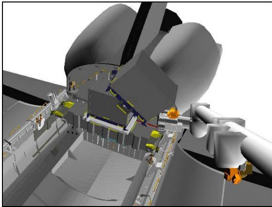
Figure 64.- APFR Uninstall (22: Base Elbow: +140, -5).
