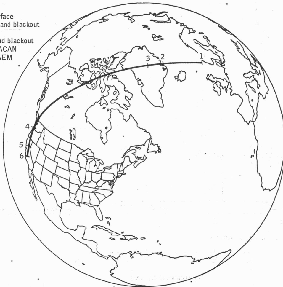
Figure 4.3-6.- Shuttle BRM 3B groundtrack from entry interface to landing.
