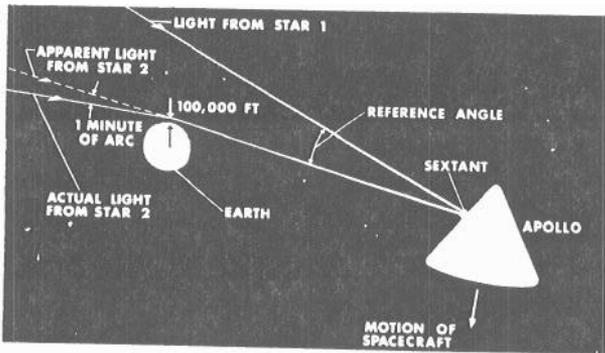
Fig. A10 Star Refraction - Earth Horizon Navigation (Reference)
