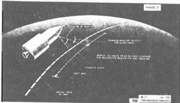
Fig. A9 S/C Orientation - Orbital Navigation (Sighting)
