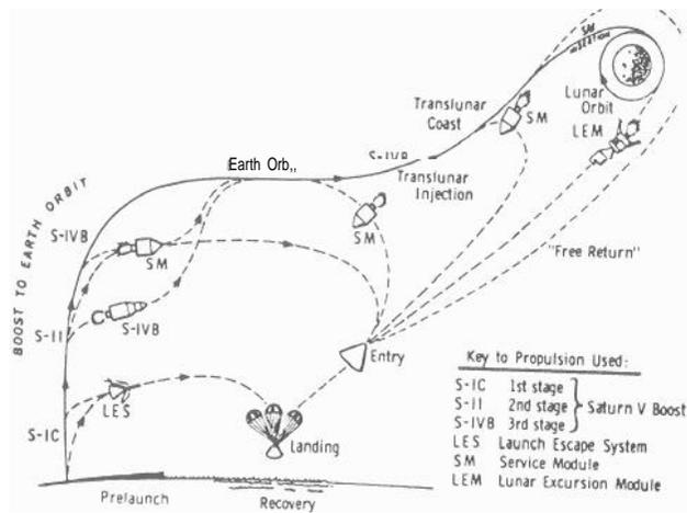
Fig. A2 Propulsion Failure Abort Paths
