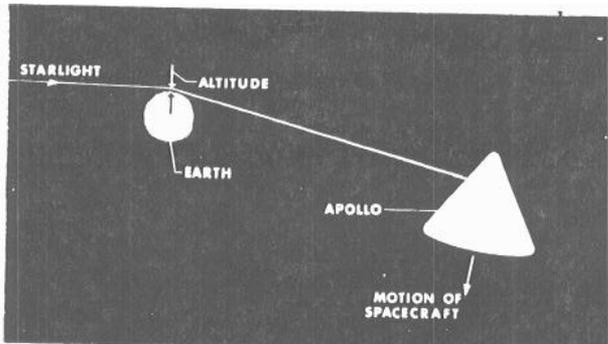
Fig. A11 Star Attenuation - Earth Horizon Navigation Reference
