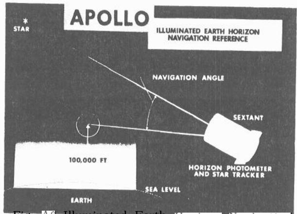
Fig. A6 Illuminated Earth Horizon Navigation Reference
