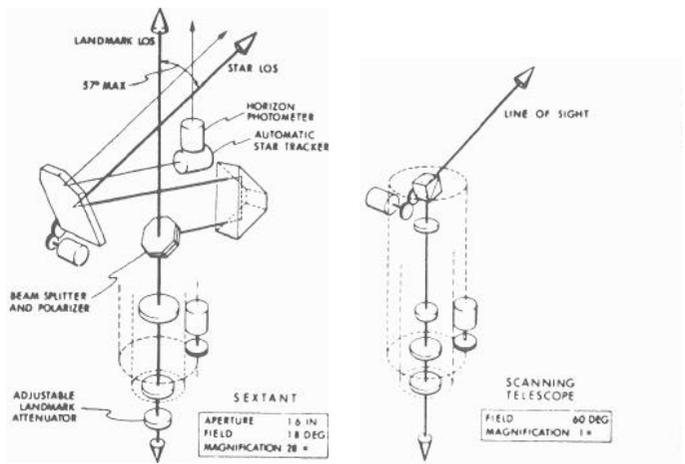
Fig. A7 Optical Schematics
