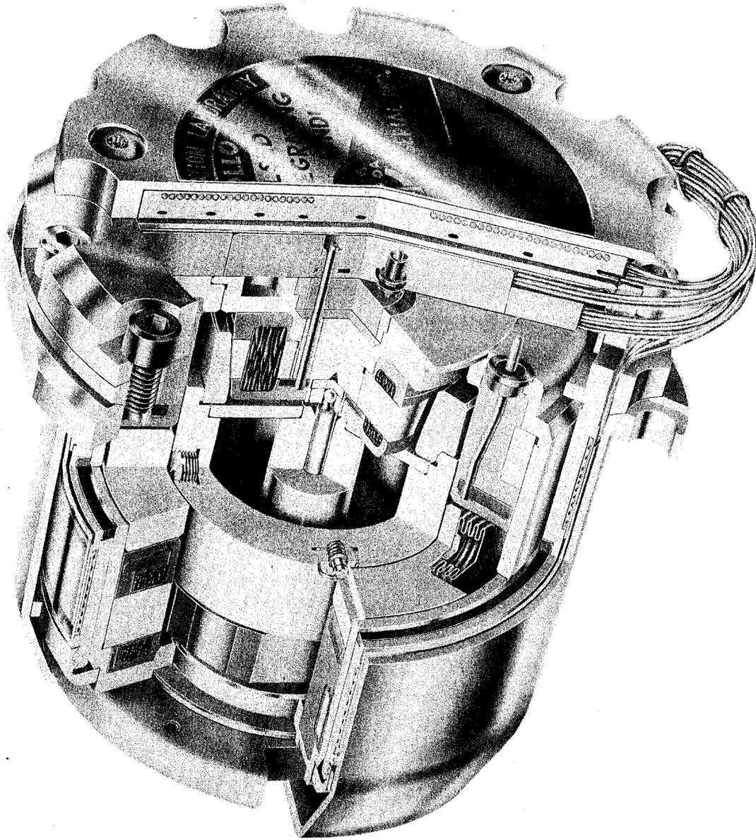
Fig. 8 16 pulsed integrating pendulum, mod D.
