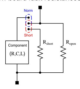
Placing jumper between upper two header pins makes the component behave normally. Placing jumper between lower two header pins emulates a partially-shorted component. Removing jumper entirely emulates a partially open component.
