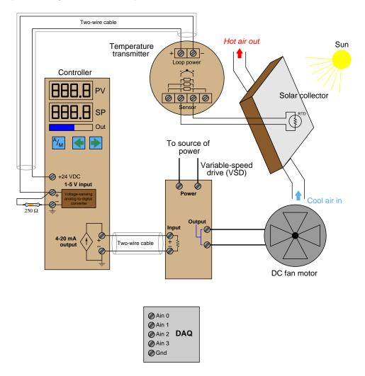
The researcher also wishes to graph the temperature and fan command signals (PV and Output) using a data acquisition module (DAQ) connecting to a personal computer. The DAQ is capable of measuring DC voltage signals ranging from 0 to +7.5 Volts (single-ended, unipolar), like a four-channel DC voltmeter sharing a common negative terminal.
