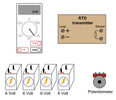
Sketch the necessary connecting wires so that the simulated RTD signal to the transmitter increases as the potentiometer's shaft is rotated (*clockwise* / *counter-clockwise*), and so that the multimeter registers the transmitter's 4-20 mA signal (using the batteries as a 24 VDC loop power supply) as a positive numerical value.
