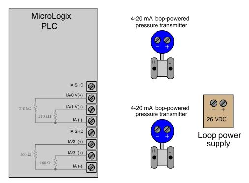
Sketch the appropriate wiring to connect one of the 4-20 mA loop-powered transmitters to current input IA/2 on the PLC, and the other transmitter to voltage input IA/0 on the PLC, using the one 26 VDC power supply to energize both.
