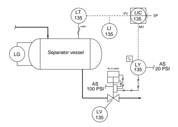
The first thing you do is look at the position of the control valve, because it is located very close to the level gauge where you and the operator are standing. You can see that the control valve is \_\_\_\_\_.
