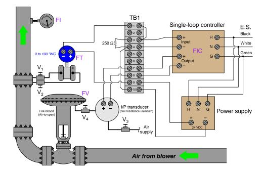
Determine the diagnostic value of each of the following tests. Assume only one fault in the system, including any single component or any single wire/cable/tube connecting components together. If a proposed test could provide new information to help you identify the location and/or nature of the one fault, mark "yes." Otherwise, if a proposed test would not reveal anything relevant to identifying the fault (already discernible from the measurements and symptoms given so far), mark "no."
