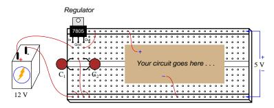
Decoupling capacitors  $C_1$  and  $C_2$  help stabilize the regulated voltage if your circuit's load current happens to pulse rather than be steady over time. Consult the regulator IC's datasheet for pin designations, recommended capacitor sizes, and also for general maximum voltage and current ratings.
