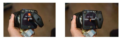
Multiple sets of switch contacts operated by the common shaft inside the lockout relay may then be used for a variety of functions, including sending trip signals to circuit breakers, activating sirens, energizing indicator lamps, sending status signals to other protective relays, inhibiting (blocking) other relay functions, etc.
