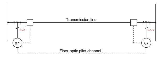
Suppose a line-to-line fault develops between phases A and B of this power line, with no connection whatsoever to earth ground. Determine whether or not the 87 relays will trip, and explain why.
