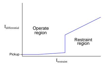
Not only may the pickup value be adjusted by the user, but also the slope of each line segment on the graph, the height of the "kneepoint" step, etc. Note how the term "restraint" is still used in digital relay configuration, even though it originated in electromechanical relay designs.
