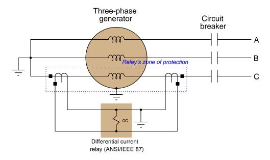
Only a fault within the relay's protection zone (i.e. an "internal" fault) is capable of forcing the two CTs currents to become unequal. Thanks to Kirchhoff's Current Law, no fault outside the protection zone (i.e. an "external" fault), no matter how severe, can make the CT primary currents become unequal<sup>3</sup>.
