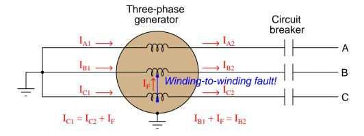
It should be noted that the magnitude of a ground fault or a winding-to-winding fault current might not be large enough to pose an overcurrent threat to the generator, yet the very existence of a current imbalance in any phase proves the winding is damaged. In other words, this is a type of system fault that would not necessarily be detected by an overcurrent (50/51) relay, and so must be detected by some other means.
