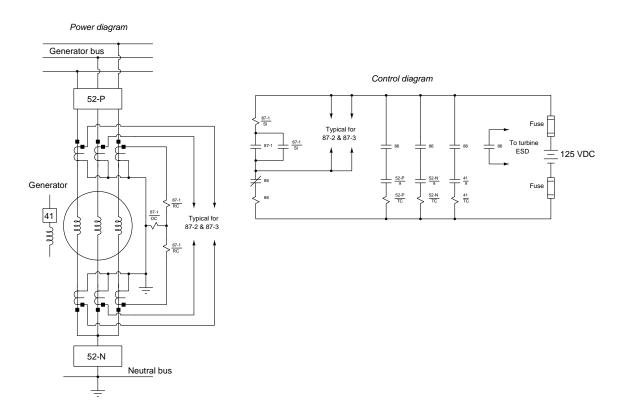
One day the auxiliary relay (86) trips for no apparent reason, which in turn trips the 52-P power breaker, the 52-N neutral breaker, the 41 field breaker, and activates the steam turbine's Emergency ShutDown system (ESD). Identify the likelihood of each specified fault for this system. Consider each fault one at a time (i.e. no coincidental faults), determining whether or not each fault could independently account for all measurements and symptoms in this circuit.
