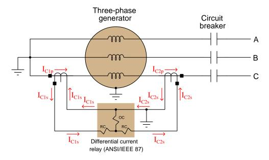
The general characteristic of a restrained differential relay is to trip on the basis of the differential current exceeding a set percentage of phase current.
