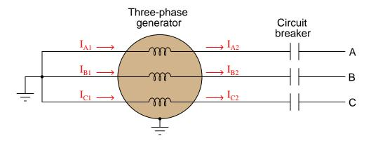
Like most large power generators, this unit brings both terminals of each phase winding to external points so that they may be connected in either a Wye or a Delta configuration as desired. In this particular case, the generator's windings are Wye-connected. So long as we measure current going in and out of each winding individually, it matters little whether those generator windings are Wye- or Delta-connected.
