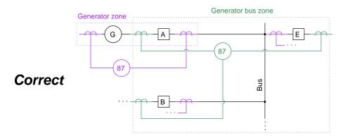
Here we see how zone overlap is achieved by connecting each differential relay to the far CT on each circuit breaker. If we instead chose to connect each 87 relay to the near CT, the two protection zones would not overlap, leaving every circuit breaker unprotected:
