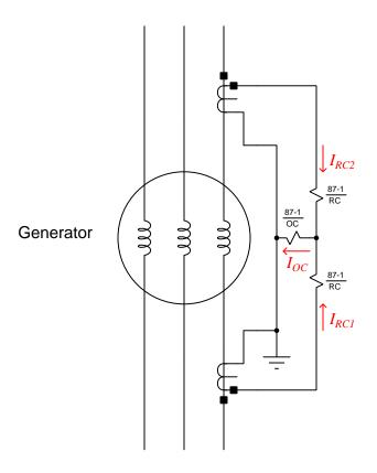
Differential current measurement is only shown here on one phase of the generator, for simplicity
