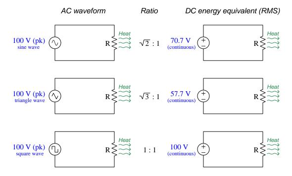
Given equal peak amplitudes, the "triangle" wave-shape is weaker than the sine wave, while a square wave is stronger than a sine wave. The differences are easy to understand if you carefully examine the wave-shapes and see which shape spends more time closer to its peak value throughout the cycle than another.
