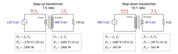
As you might imagine, an electrical component having no moving parts that is able to convert high-voltage to low-voltage (and vice-versa) is very useful, especially for electrical power systems. The fact that these devices require AC and cannot function on DC is one of the most significant historical reasons why AC triumphed over DC for electrical power distribution.
