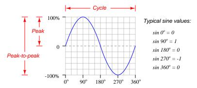
By definition, one *cycle* of a wave is 360 degrees of revolution, during which the wave will reach both a positive peak value as well as a negative peak value. *Peak* value, in fact, is a simple method of quantifying AC amplitude. Sometimes it is useful to express an AC quantity in terms of its over-all wave height from positive peak to negative peak, and we call this the *Peak-to-Peak* amplitude of the wave.
