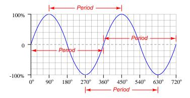
Period is typically measured in seconds, and the reciprocal of period is called frequency(f) which used to be measured in  $cycles\ per\ second$  (cps) but now has its own unit of the  $Hertz\ (Hz)^4$ . For example, in many parts of the world the standard frequency for AC power systems is 60 Hz, equating to a period of 16.67 milliseconds. In other parts of the world the standard frequency for AC electric power is 50 Hz, with a period of 20 milliseconds.
