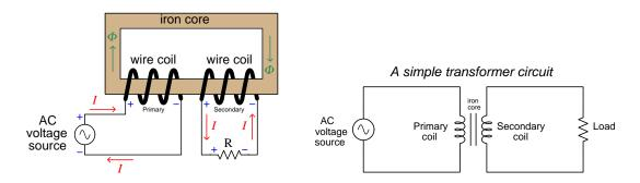
If the electrical source energizing the first ("primary") coil outputs a varying current, the magnetic field produced by that coil must vary as well, and this variation over time *induces* voltage in the second ("secondary") coil as described by Faraday's Law of Electromagnetic Induction:
