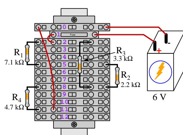
Numbering on the terminal blocks provides a very natural translation to SPICE<sup>10</sup> netlists, where component connections are identified by terminal number:
