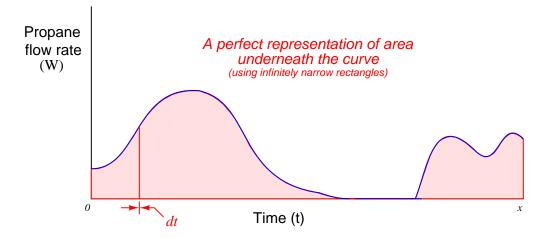
If we represent infinitesimal time increments using the notation "dt" as opposed to the notation " $\Delta t$ " used to represent discrete time periods, we must also use different notation to represent the mathematical sum of those quantities. Thus, we will replace the "sigma" symbol ( $\Sigma$ ) used for summation and replace it with the integral symbol (f), which means a *continuous* summation of infinitesimal quantities:
