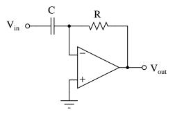
$$V_{out} = -RC\frac{dV_{in}}{dt}$$
