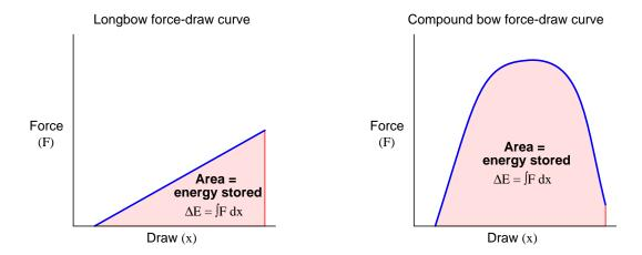
This is why a compound bow is so much more powerful than a longbow or a "recurve" bow with the same holding force: the energy represented by the greater area underneath the force-draw curve equates to greater energy imparted to the arrow when released, and therefore greater kinetic energy in the arrow during flight.
