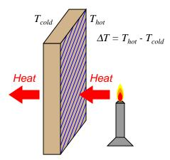
Once again,  $\Delta T$  is calculated by subtracting one temperature from another. Here, the sign (positive or negative) of  $\Delta T$  denotes the *direction* of heat flow through the thickness of the wall.
