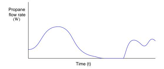
The physics of gas flow and gas mass over time has not changed: *total propane mass consumed* over time must still be the area enclosed beneath the flow curve. The only difference between this example and the two previous examples is the complexity of actually calculating that enclosed area.
