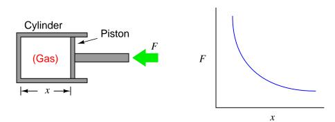
A more sophisticated example of numerical integration used to calculate work is that of a heat engine, where a piston compresses an enclosed gas:
