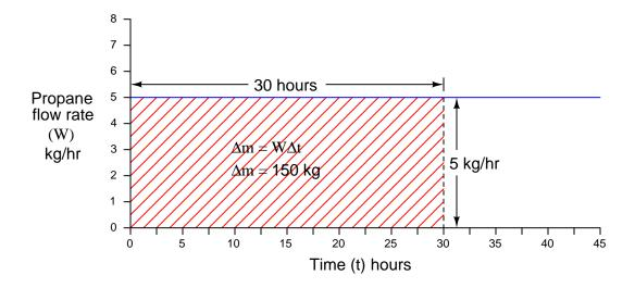
To summarize: the height of this graph represents the rate at which propane exits the storage tank, the width of the graph represents the length of time propane has been consumed from the storage tank, and the geometric area enclosed by these two boundaries represents the total mass of propane consumed during that time. Height in *kilograms per hour* multiplied by width in *hours* equals *kilograms*.
