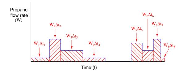
Each rectangular area underneath the flow line on the graph  $(W_n \Delta t_n)$  represents a quantity of propane gas consumed during that time period. To find the total amount of propane consumed in the time represented by the entire graph, we simply sum these mass quantities together:
