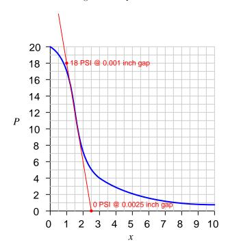
Choosing convenient points<sup>18</sup> on this tangent line aligning with major divisions on the graph's scales, we find two coordinates we may use to calculate the derivative of the curve at its steepest point:
