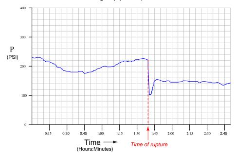
An example of a modern<sup>11</sup> pressure-trend recording during a pipeline rupture is shown here:
