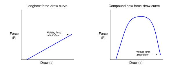
The force required to draw a compound bow rises sharply during the first few inches of draw, peaks during the region where the archer's arms are ideally angled for maximum pulling strength, then "lets off" toward the end where the archer's drawing arm is weakest in the "holding" position. The result is a bow that requires substantial force to draw, but is relatively easy to hold in fully-drawn position.
