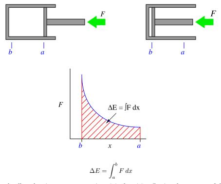
If we slowly allow the piston to return to its original position (letting the pressure of the enclosed gas push it back out), the piston's force decreases as displacement increases. The force/displacement relationship is the same as before, the only difference being the direction of travel is opposite. This means the change in energy is happening over the same interval, in reverse direction (from b to a now instead of from a to b). Expressed as an integral:
