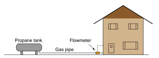
By measuring true mass flow rate, it should be possible to indirectly measure how much propane gas has been consumed at any time following the most recent filling of the tank. For example, if the mass flow rate of propane out of the tank happened to be a constant 5 kilograms per hour for 30 hours straight, it would be a simple matter of multiplication to calculate the consumed mass:
