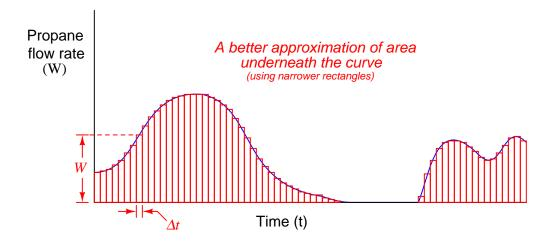
Taking this idea to its ultimate realization, we could imagine a super-computer sampling mass flow rates at an infinite speed, then calculating the rectangular area covered by each flow rate (W) times each infinitesimal increment of time (dt). With time increments of negligible width, the "approximation" of area underneath the graph found by the sum of all these rectangles would be perfect – indeed, it would not be an approximation at all, but rather an exact match:
