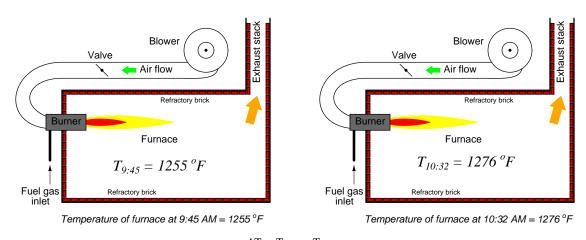
For example, if the temperature of a furnace (T) increases over time, we might wish to describe that change in temperature as  $\Delta T$ :
