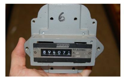
The fact that this instrument's display resembles the odometer of an automobile is no coincidence. Odometers are really just another form of mechanical integrator, "totalizing" the distance traveled by a vehicle. If the speedometer of a vehicle registers speed (v) in units of miles per hour, then the odometer will accumulate a distance  $(\Delta x)$  in units of miles, since distance (miles) is the time-integral of speed (miles per hour):
