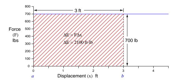
Lifting the mass vertically constitutes a *positive* change in potential energy for this object, because each displacement differential (dx) is a positive quantity as we move from a height of 0 feet to a height of 3 feet:
