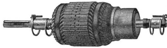
FIG. 400.—Fairbanks-Morse armature for 7½ H. P., 1300 R. P. M., TR type motor. The armature core is built up of thin sheet steel laminations with notches in the circumference, which, when the discs are placed together, form grooves or slots to receive the armature coils. The armature cores for the larger machines are mounted on a cast iron spider, which also carries the commutator, making the two parts entirely self-contained, and with this construction, it is possible to remove the armature shaft, without disturbing the core, commutator or windings. Cores of all sizes are provided with ventilating spaces, running from the surface to the central opening of the core, so that air is drawn through the core and blown out over the windings by the revolution of the armature.
