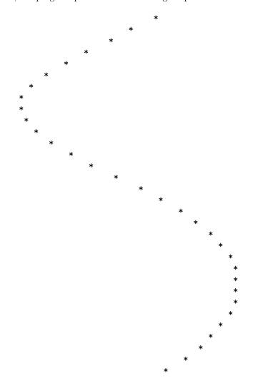
As you can see, the waveform is not a perfect sinusoid. This is due to the nonlinear nature of the FET, being a square-law device.
