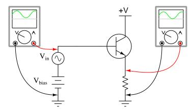
This amplifier's output signal faithfully represents the wave-shape of the AC input signal, and is also "biased" above zero as a result of the transistor being incapable of controlling a bidirectional current.
