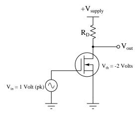
The FET used in this example is a depletion-type N-channel MOSFET with a turn-off (i.e. threshold) voltage of -2 Volts. The input voltage source is AC with a peak value of 1 Volt, which means it alternates in sinusoidal fashion reaching peak instantaneous voltage values of +1 Volt and -1 Volt. Thus, the input voltage source will never reach a value large enough to fully turn off the MOSFET – it will always remain conductive between drain and source.
