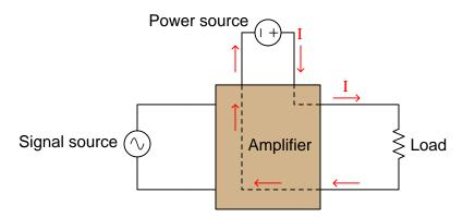
Electronic components such as transistors (or, in previous eras, vacuum tubes) comprise the heart of amplifiers, giving the input signal control over the flow of energy from power source to load.
