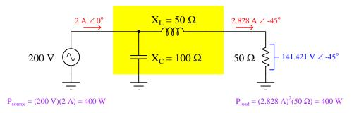
Note how with the simple LC network the source "sees" a 100 Ohm load impedance even though the actual load is 50 Ohms, and also how load power and source power are precisely equal (at least given an ideal inductor and an ideal capacitor having no dissipative losses).
