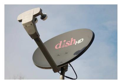
The rationale for having three LNBs offset from one another is to be able to receive signals from three different satellites in geosynchronous orbit without re-positioning the directional dish antenna.
