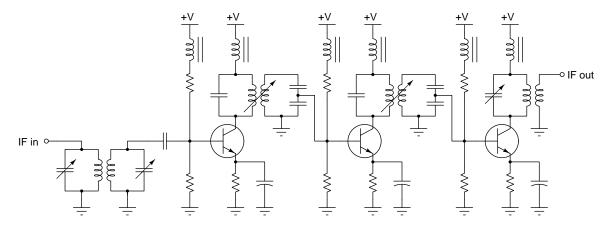
The procedure to adjust all these double-tuned tank circuits for optimum IF amplifier performance is called alignment, or sometimes  $peaking^6$ .
