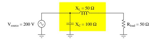
If we perform the necessary series-parallel impedance calculations for the LC network and resistive load, we find that the total impedance (as calculated from the perspective of the input terminal where the source would connect) is precisely 100 Ohms resistive (i.e.  $100 \Omega \angle 0^{\circ}$  or 100 + j0) which is twice the impedance of the load with the same phase angle.
