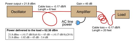
A similar application of decibels is found in multi-stage amplifier circuits, where one stage amplifies a signal to be fed into a successive stage to be amplified more. The power gains of these stages, each expressed as a ratio, multiply to make the over-all amplifier's power gain (ratio). The power gains of those same stages, each expressed as a decibel figure, add to make the over-all amplifier's power gain (dB):
