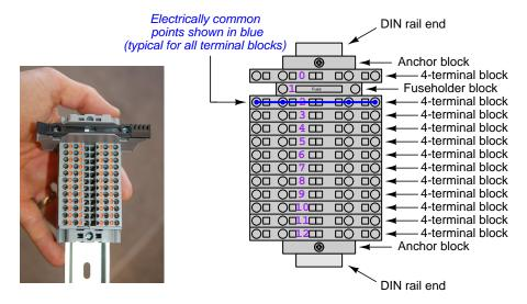
Screwless terminal blocks (using internal spring clips to clamp wire and component lead ends) are preferred over screw-based terminal blocks, as they reduce assembly and disassembly time, and also minimize repetitive wrist stress from twisting screwdrivers. Some screwless terminal blocks require the use of a special tool to release the spring clip, while others provide buttons<sup>9</sup> for this task which may be pressed using the tip of any suitable tool.
