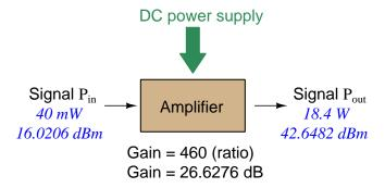
Notice how the output and input powers expressed in dBm relate to the power gain of the amplifier. Taking the input power and simply *adding* the amplifier's gain factor yields the amplifier's output power in dBm:
