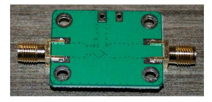
$<sup>^{2}</sup>$ In PCB layout terminology, a via is a metal-plated hole designed to electrically connect copper traces or planes on different layers of the printed circuit board.
