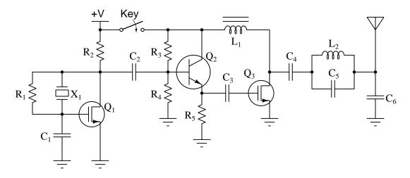
Identify the effects of the following faults in this transmitter:
