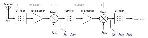
Amplifier design becomes more complicated as frequency increases, which is good design rationale for the existence of IF signals and IF amplifiers: downconvert the RF signal into a more manageable frequency range, then amplify it there rather than try to do so at the extremely high frequencies of RF.
