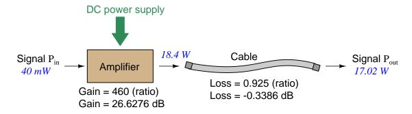
The overall gain of this amplifier and cable system expressed as a ratio is equal to the *product* of the individual component gain/loss ratios. That is, the gain ratio of the amplifier *multiplied* by the loss ratio of the cable yields the overall power ratio for the system:
