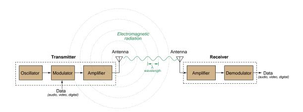
In the block diagram shown above, the two amplifiers operate at the same frequency but at radically disparate power levels. The transmitter's RF amplifier must output fairly high power to effectively radiate electromagnetic waves from its antenna. The receiver's RF amplifier must amplify the incredibly weak RF signal captured by its antenna without contributing much noise to that signal.
