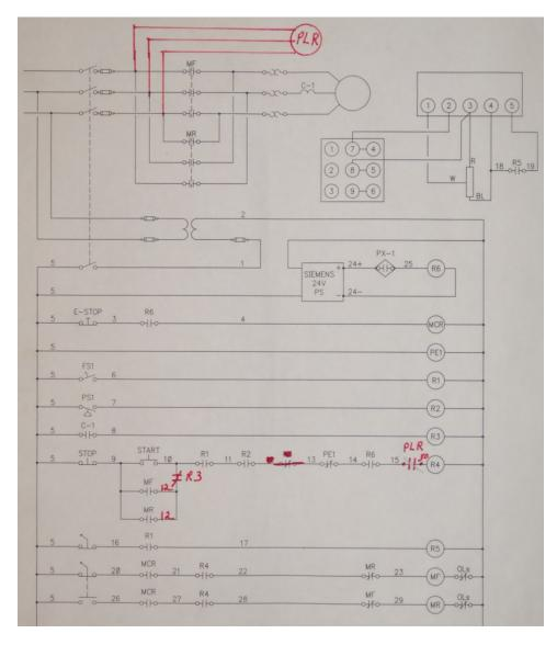
The red-lined edits made to this diagram show a *power loss relay* (PLR) added to the motor circuit, designed to interrupt power to control relay R4 in the event of a loss of three-phase electrical power. Also changed in this diagram is the location of the normally-closed contact R3, which is actuated by overload relay C-1.
