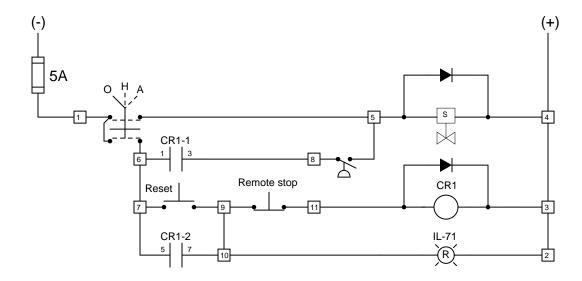
Suppose the solenoid valve refuses to energize when the Hand/Off/Auto switch has been placed in "Auto," the Reset pushbutton pressed, and a high-pressure condition exists. The solenoid can, however, be made to energize by placing the switch in the "Hand" position.
