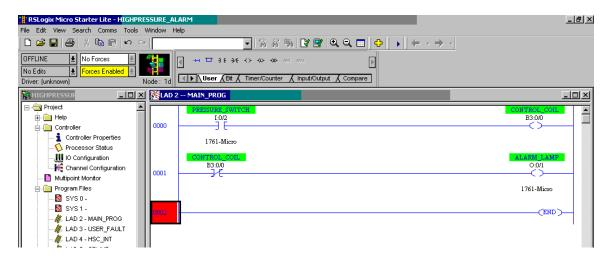
Suppose a fluid pressure of 36 PSI is applied to the pressure switch. This is less than the switch's trip setting of 50 PSI, leaving the switch in its "normal" (closed) state. This sends power to input I:0/2 of the PLC. The contact labeled I:0/2 drawn in the ladder-logic program of the PLC acts like a relay contact driven by a coil energized by input terminal I:0/2. Thus, the closed pressure switch
