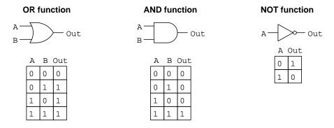
By combining OR and AND functions with inversion (the NOT function), we may form two more common "building-block" logical functions, NOR and NAND:
