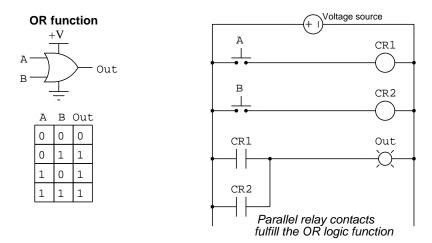
This ladder-style diagram is so much clearer than the schematic-style diagram previously shown, owing to the complete absence of any crossing lines. The parallel connection between the two relays' normally-open contacts is quite obvious in the ladder diagram, and the lack of dashed lines connecting relay contacts to their respective coils unclutters the illustration.
