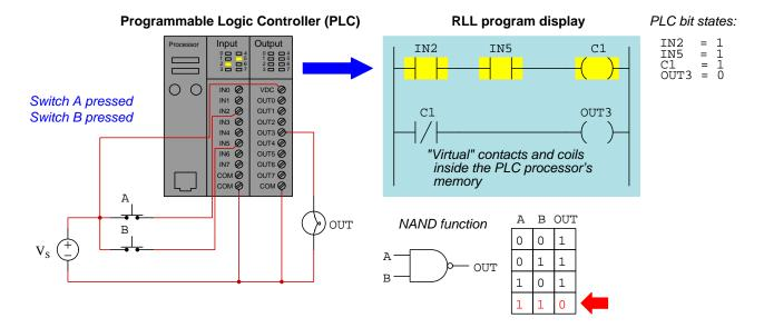
"Ladder-logic" programming is limited compared to text-based computer programming languages, but it is far more intuitive and resembles the diagrams of relay control systems PLCs were designed to replace. Some modern PLCs support text-based and function-block-based programming languages in addition to RLL, in order to give the end-user an array of programming options.
