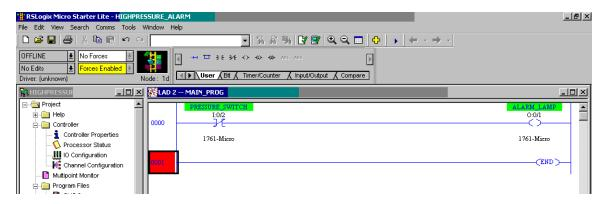
The effect is the same: the PLC output 0:0/1 will activate whenever input I:0/2 de-energizes (whenever the pressure switch is opened by a high pressure), turning on the alarm lamp in a high-pressure condition. In a low-pressure condition, the energized input I:0/2 forces the virtual normally-closed contact I:0/2 to open, thus de-energizing the PLC's output 0:0/1 and turning the alarm lamp off.
