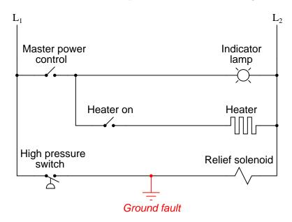
What would be the result of this ground fault? Would it matter if the L1/L2 power connections were reversed?
