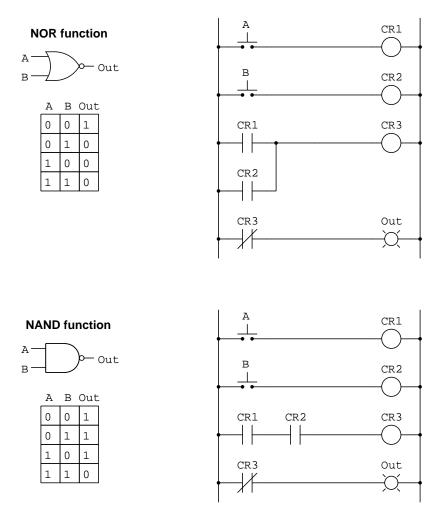
It is very important to realize that the diagonal line drawn through a relay contact represents its *normal state* and not necessarily its *present state* or *typical state*. In fact, this is one of the most common misconceptions for students first encountering ladder diagrams.
