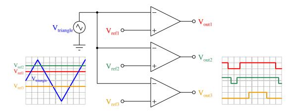
If there is a need for either the rising or the falling edges of these PWM signals to all be synchronized, simply replacing the triangle-wave signal with a ramp signal will ensure this happens:
