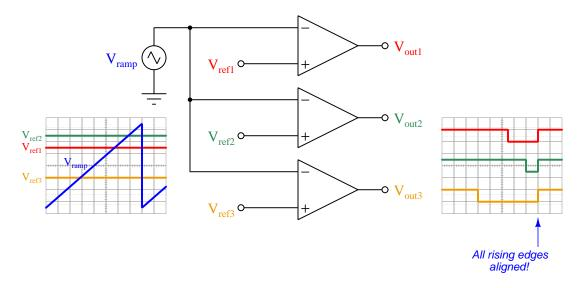
In the example shown above, the gradual climb and rapid fall of the ramp waveform ensures alignment of the PWM pulses at their falling edges. If we wished the PWM pulses to be aligned at their rising edges instead, we could substitute a ramp waveform that rises rapidly and falls gradually.
