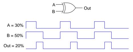
In this example signal A has a duty cycle of 30% while signal B has a higher duty cycle of 50%. Both signals have their rising edges<sup>7</sup> synchronized, and when this condition is met the resultant output signal's duty cycle will be the *absolute value of the difference* between the two inputs'.
