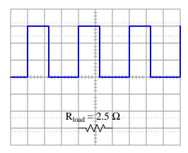
Vertical sensitivity = 1 Volt/div Probe ratio = 1:1 Coupling = DC Timebase = 0.5 ms/div
