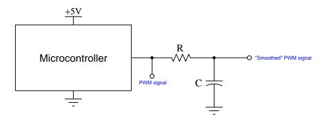
Many microcontrollers and other programmable devices have only digital (discrete high/low) output signal capability, and so if an analog output signal is desired the "smoothed" PWM technique may be a valid solution. As you can see, the filtered signal is not a perfect sawtooth waveform, but it may be close enough depending on the application.
