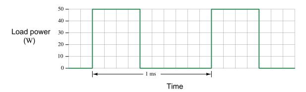
We already know that the average power in this case must be 20 Watts because the peak power is 50 Watts and the duty cycle is 40%. Let's dissect this scenario a bit more, though, to explore why this is the case. Our first step is recognizing the definition of power, which is the rate of energy transfer over time. In fact, 1 Watt of power is defined as 1 Joule of energy transferred from one location to another over a time of 1 second; i.e. Watts is equal to Joules per second.
