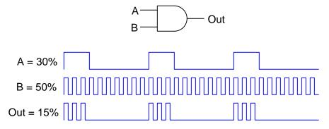
Here, the 50% duty-cycle signal makes it so the 30% duty-cycle signal is "high" only for half the amount of time it would have been without the influence of the AND gate, thereby scaling down signal A's duty cycle of 30% to a mere 15%. What we see here is *multiplication* of duty cycle values, with the output signal's duty cycle being the product of the two input signals' duty cycles:
