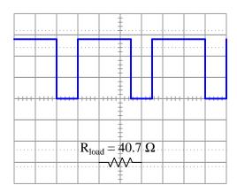
Vertical sensitivity = 5 Volts/div Probe ratio = 10:1 Coupling = DC Timebase = 0.2 ms/div
