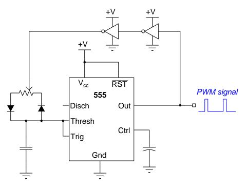
Which way should you move the potentiometer's wiper to increase duty cycle?
