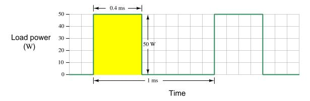
Since we know power is energy divided by time (i.e. Watts equals Joules per second), then it must be true that energy is power multiplied by time (i.e. Joules equals Watts *times* seconds). Having labeled the height and width of one of the "high" pulse durations, we may determine the geometric area of that enclosed rectangle as the product of power and time. As we show here, 50 Watts multiplied by 0.4 milliseconds is 20 milliJoules of energy:
