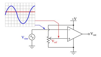
Assuming the same 3 Volt peak amplitude for the sine wave, calculate the necessary  $V_{ref}$  to generate the following duty cycle values:
