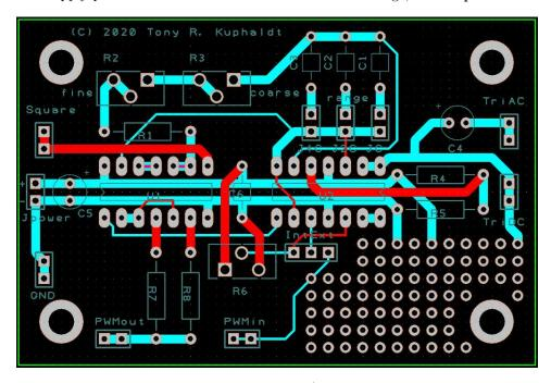
Note how two pads are provided for each of the I/O terminals. This was done to facilitate a small loop of bare wire soldered between the two pads, which makes an easy connection point for "grabber" hooks or "alligator" clips. The four large pads at the board's corners are intended for nylon stand-offs, for mounting this PCB to a larger panel. These mounting pads are spaced 2.5 inches horizontally and 1.5 inches vertically from each other.
