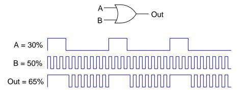
Here, the higher-frequency signal with its 50% duty cycle controls the output when the lower-frequency signal is "low", but when the lower-frequency signal is "high" it completely overrides the other signal to force the output high for that same duration of time. In other words, the aggregate duty cycle for the OR gate's output signal will be 30% (from the A signal) plus 50% of the A signal's complement (50% of 70% = 35%). Generalized in mathematical form:
