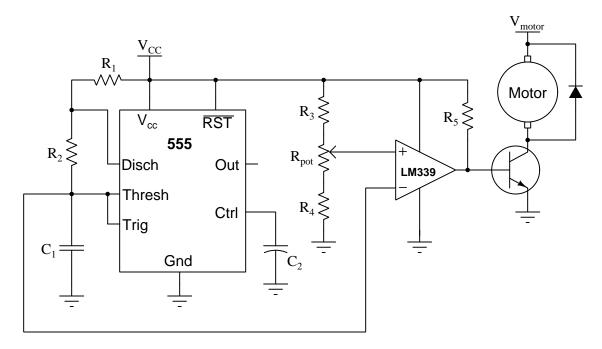
Here it is imperative to properly size resistor  $R_5$  since it must supply adequate current to the transistor's base to saturate it in the "on" state. Too large of a value for  $R_5$  will cause the transistor to not turn on fully, dropping excessive  $V_{CE}$  and dissipating excessive power in the form of heat; too small of a value for  $R_5$  will force the LM339 comparator to have to sink too much current, possibly overstressing it.
