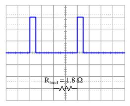
Vertical sensitivity = 20 Volts/div Probe ratio = 1:1 Coupling = DC Timebase = 0.1 ms/div
