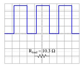
Vertical sensitivity = 1 Volt/div Probe ratio = 10:1 Coupling = DC Timebase = 20  $\mu$ s/div
