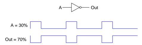
In this example, we see an input PWM signal with a duty cycle of 30% get converted into an output PWM signal with a duty cycle of 70%. Those two percentages, being complementary to each other, when added together must equal 100%.
