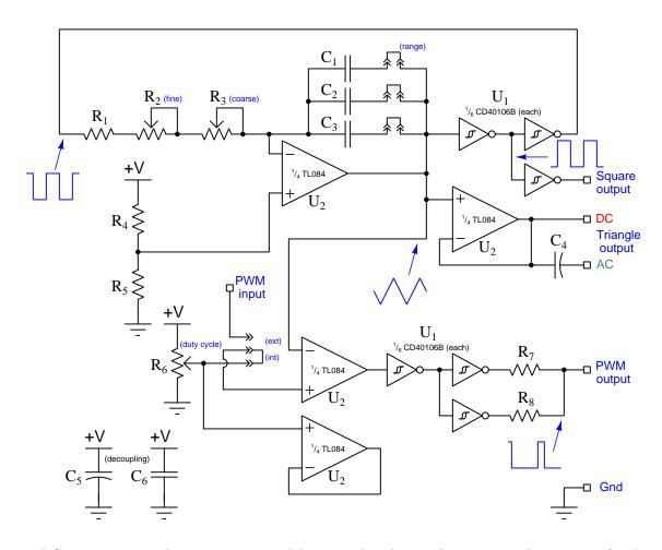
DC power source voltage may range widely, given the advertised operating voltage ranges for the CD40106B and TL084 integrated circuits (3 to 18 Volts for the hex inverter and 10 to 30 Volts for the opamp). I have successfully tested this circuit at a supply voltage as low as 5 Volts and it seems to work well.
