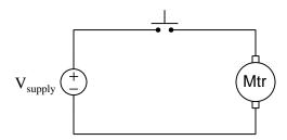
The motor will run any time the switch is pressed, because pressing the pushbutton causes its contacts to close and complete the circuit. Releasing the switch causes its contacts to return to their "normal" (resting) state and breaks the circuit. What could be simpler than this?
