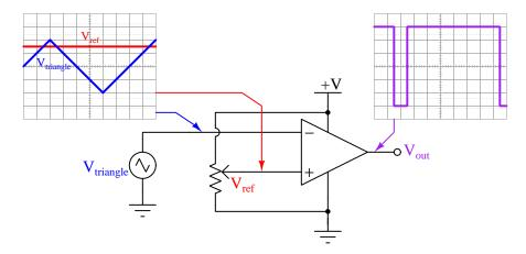
Whenever  $V_{ref}$  exceeds  $V_{triangle}$ , the comparator's output goes "high" (on for any ground-referenced load); whenever  $V_{ref}$  is less than  $V_{triangle}$ , the output goes "low" (off for any ground-referenced load). The higher  $V_{ref}$ , the longer the output remains "high" and the shorter it remains "low" during the cycle. Thus, the amplitude of  $V_{ref}$  determines the duty cycle of the pulse output, while the frequency is set by the frequency of the triangle-wave source.
