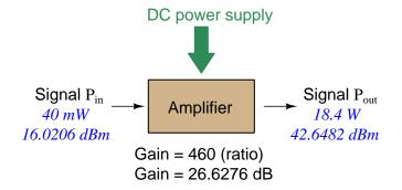
Notice how the output and input powers expressed in dBm relate to the power gain of the amplifier. Taking the input power and simply *adding* the amplifier's gain factor yields the amplifier's output power in dBm:
