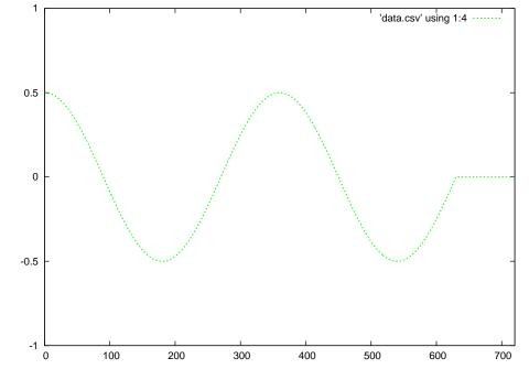
$\mbox{Green} = \mbox{superposition}$  of the forward and reflected waves
