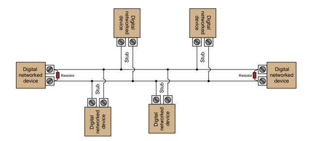
Note that the far-end devices have terminating resistors connected in parallel to the network connection terminals, while the devices at the end of the stubs do not. Does this constitute a problem? In other words, will reflected signals result from the unterminated stubs? Why or why not?
