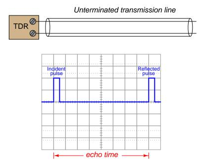
Write a formula relating echo time (t), cable length (x), and velocity factor (k) together.
