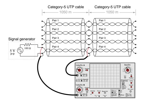
$<sup>^{4}</sup>$ One detail that might be worth mentioning is that the oscilloscope would have to have isolated inputs in order for this test to work. Otherwise, the common ground connection through both inputs (A and B) would mess things up by bypassing one wire in the twisted pair with the first 1050 meter section!
