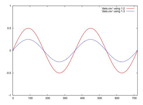
After the reflected wave has traveled all the way back to the source (left-hand end of the transmission line), the superposition of those two continuous waves results in a standing wave.
