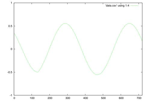
$\mbox{Green}=\mbox{superposition}$  of the forward and reflected waves
