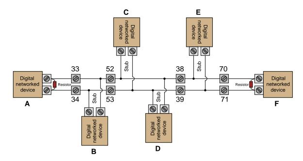
The technician decides to loosen terminal number 38 and remove the wire entering its lefthand side. Then, she uses her ohmmeter to measure resistance between terminals 52 and 53. The ohmmeter registers 152 Ohms.
