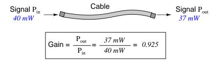
$$10\log\left(\frac{P_{out}}{P_{in}}\right) = 10\log\left(\frac{37 \text{ mW}}{40 \text{ mW}}\right) = -0.3386 \text{ dB}$$
