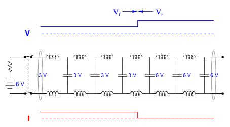
We know the open creates a full-voltage condition at the line's far end, and over time this becomes a full-voltage condition along the entire line. If we view that final condition as the *superposition* of the forward and reflected pulses, it means the reflected voltage pulse has the same polarity (i.e. 0 degrees out of phase) as the forward pulse in order to double the forward pulse's magnitude. This means  $V_r = V_f$ , which means the line's reflection coefficient must be positive one:
