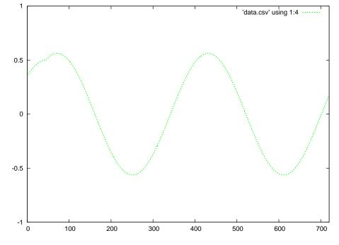
$\mbox{Green} = \mbox{superposition}$  of the forward and reflected waves
