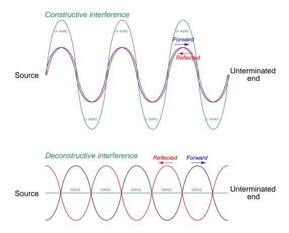
This phenomenon is known as a *standing wave*: regions of high alternating amplitude and low (or zero) amplitude that do not travel along the line in the same manner as either the forward or reflected wave but rather "stand still". To see a flip-book animation of how standing waves form, refer to section 5.4 beginning on page 99.
