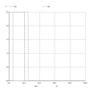
In this simulation voltage source  $V_1$  outputs a 5-Volt pulse lasting 20 nanoseconds, which is seen at the far end of the transmission line (voltage between nodes 3 and 0) 5 ns later. The voltage between nodes 2 and 0 only goes to 2.5 Volts (not 5 Volts) because the transmission line acts as a 50-Ohm load. Proper termination ensures there is no reflection, and so we see the same 2.5 Volt pulse at the far end and no interference back at the source end.
