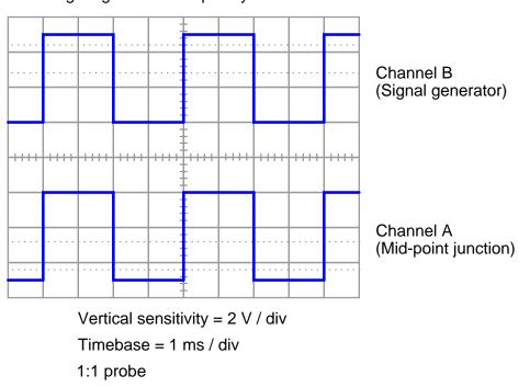
Signal generator frequency = 250 Hz
