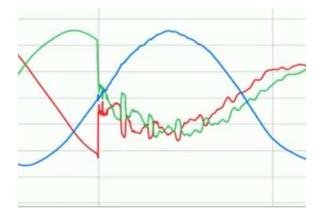
A series of impulses are clearly visible immediately after the fault's onset, created as the pulses echo back and forth between the substation (where the oscillography equipment was located) and the fault location. Assuming a 60 Hz power line frequency and a velocity factor of 95% for open-air power lines, approximate the distance between the substation and the fault.
