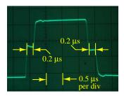
This particular cable has a *velocity factor* of approximately 0.7, which means electrical impulses travel only 70% as fast as light travels through a vacuum, and so the round-trip distance based on that echo propagation time is approximately 42 meters:
