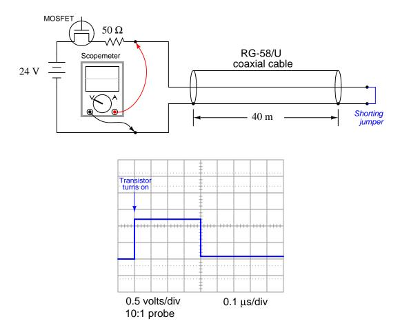
Again, explain why the voltage waveform does this. Why doesn't the voltage remain nearly zero the entire time, given a dead short at the end of the cable?
