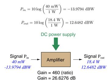
Note how the input power of 40 milliWatts equates to a negative dBW figure because 40 milliWatts is *less* than the 1 Watt reference, and how the output power of 18.4 Watts equates to a positive dBW figure because 18.4 Watts is *more* than the 1 Watt reference. A positive dB figure means "more than" while a negative dB figure means "less than."
