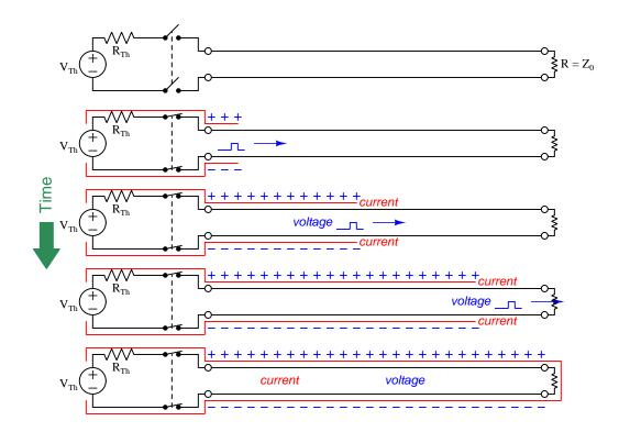
From the perspective of the pulse source, this properly terminated transmission line "looks" the same as an unterminated line of infinite length. There is no reflected pulse, and the DC voltage source "sees" an unchanging load resistance the entire time.
