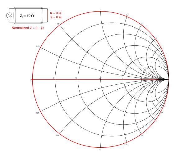
This is the point marked by the intersection of a full-radius resistance circle and a reactance circle having an infinite radius (i.e. a "circle" which is really a straight line overlapping the horizontal axis).
