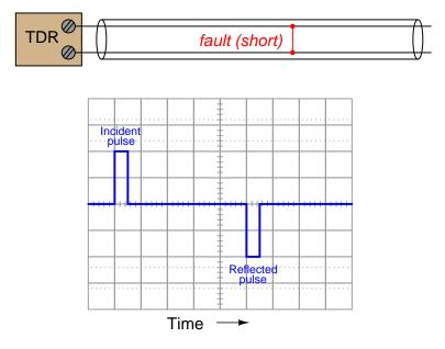
What would the technician look for in the TDR display to determine where the fault was in the cable? Also, what would the TDR display look like for a good (non-faulted) cable?
