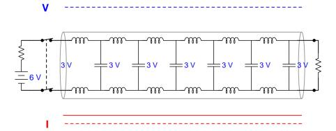
In this case, the reflection coefficient must be equal to zero as well:
