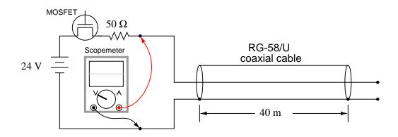
The characteristic impedance of an RG-58/U cable is 50  $\Omega$  (also called the "surge" impedance), and the Thévenin equivalent impedance of our power supply is 50  $\Omega$  as well. When the transistor is turned on, the scope registers an immediate step in voltage, but only to 12 Volts (one-half the supply voltage). It isn't until several tenths of a microsecond later that the voltage steps up to the full 24 Volts:
