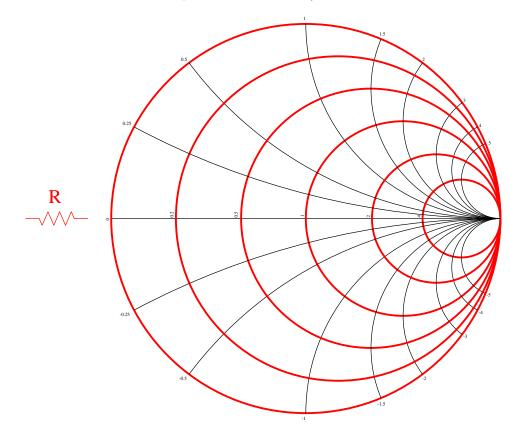
The reactance circles of a Smith chart lie along the vertical axis and intersect at the far-right end of the horizontal axis, each one having a radius proportional to  $\frac{1}{X}$  where X is the *normalized* reactance of the terminating impedance (i.e. the terminating impedance's reactance value divided by the transmission line's characteristic impedance value of 50  $\Omega$ ):
