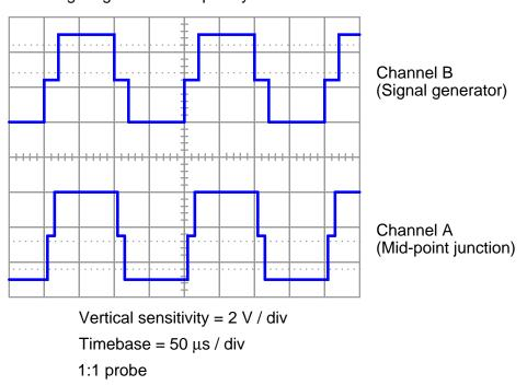
Signal generator frequency = 5 kHz
