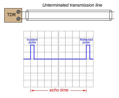
Build a computer spreadsheet to calculate cable length, given the echo time (entered in microseconds) measured by a TDR, and the velocity factor of the cable. An example spreadsheet layout is shown here (the cell fill coloring is just for looks, distinguishing the *calculated* value of cable length from the *entered* values of echo time and velocity factor):
