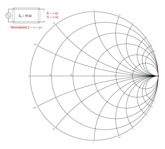
This is the point marked by the intersection of a zero-radius resistance circle and a zero-radius reactance circle.
