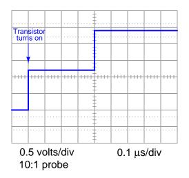
Explain why the voltage waveform steps to 12 Volts, then to 24 Volts as it does. Why doesn't it step all the way to 24 Volts immediately, given a cable that is open at the far end?
