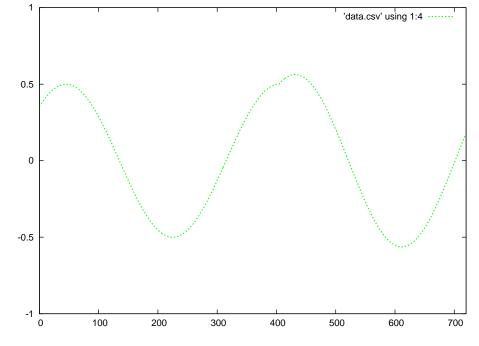
Green = superposition of the forward and reflected waves
