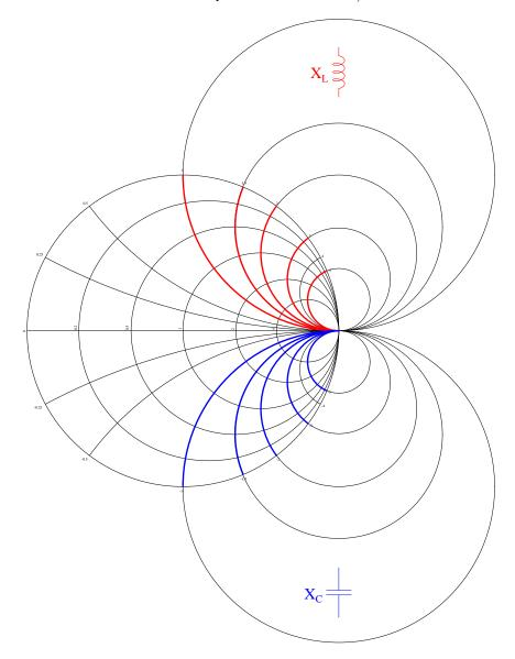
Inductive reactance values are positive (above the horizontal axis) while capacitive reactance values are negative (below the horizontal axis).
