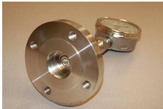
The only difference between this chemical-seal gauge and a remote-seal gauge is that a remote-seal gauge uses a length of very small-diameter tubing called *capillary tubing* to transfer fill fluid pressure from the sealing diaphragm to the gauge mechanism.
