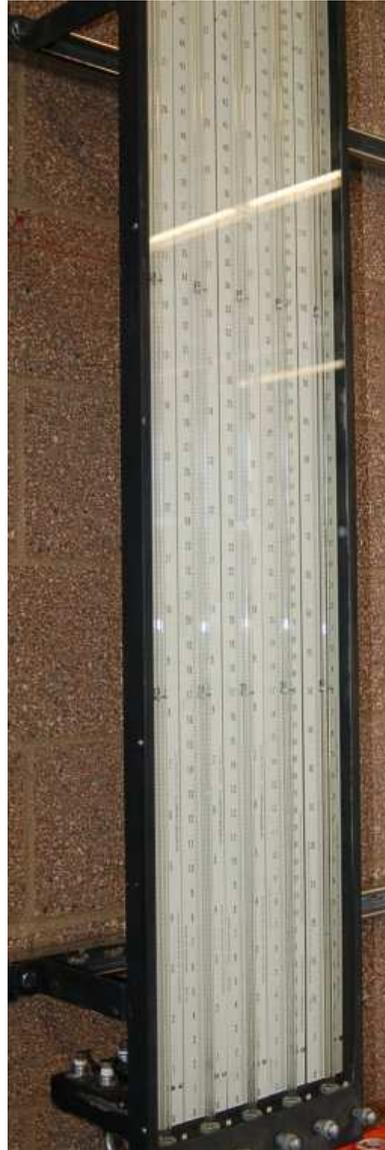
Inclined manometers are used to measure very low pressures, owing to their exceptional sensitivity (note the fractional scale for inches of water column in the following photograph, extending from 0 to 1.5 inches on the scale, reading left to right):
