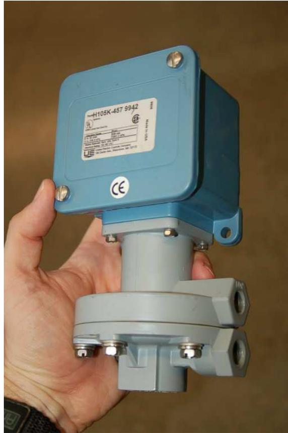
The electrical switch element is located underneath the blue cover, while the diaphragm pressure element is located within the grey metal housing. The net force exerted on the diaphragm by the two fluid pressures varies in magnitude and direction with the magnitude of those pressures. If the two fluid pressures are precisely equal, the diaphragm experiences no net force (zero differential pressure).
