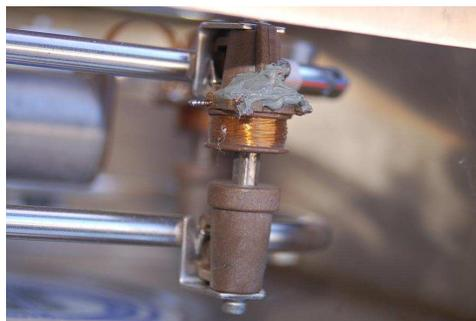
Advances in sensor technology and signal processing have allowed the construction of Coriolis flowmeters employing straighter tubes than the U-tube unit previously illustrated and photographed. Straighter tubes are advantageous for reasons of reduced plugging potential and the ability to easily drain all liquids out of the flowmeter when needed.
