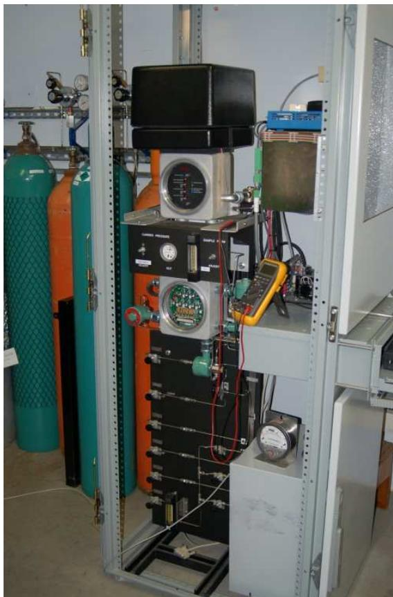
This particular GC is used by a natural gas distribution company as part of its pricing system. The heating value of the natural gas is used as data to calculate the selling price of the natural gas (dollars per standard cubic foot), so that the customers pay only for the actual benefit of the gas (i.e. its ability to function as a fuel) and not just volumetric or mass quantity.
