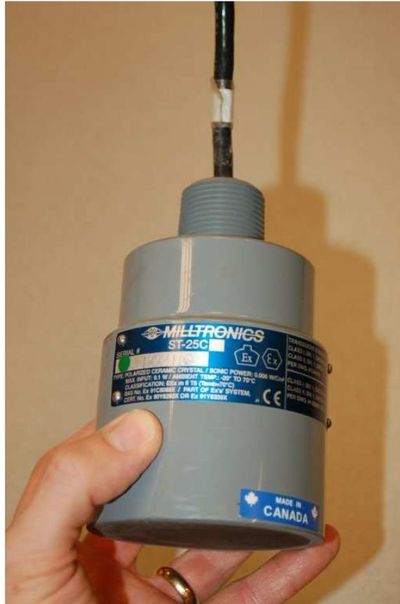
If the ultrasonic transducer is rugged enough, and the process vessel sufficiently free of sludge and other sound-dampening materials accumulating at the vessel bottom, the transducer may be mounted at the bottom of the vessel, bouncing sound waves off the liquid surface through the liquid itself rather than through the vapor space:
