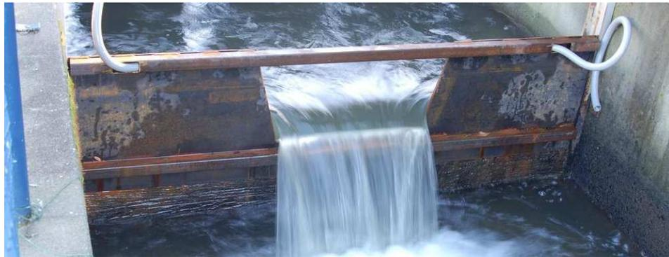
At a condition of zero flow through the channel, the liquid level will be at or below the crest (lowest point on the opening) of the weir. As liquid begins to flow through the channel, it must spill over the crest of the weir in order to get past the weir and continue downstream in the channel. In order for this to happen, the level of the liquid upstream of the weir must rise above the weir's crest
