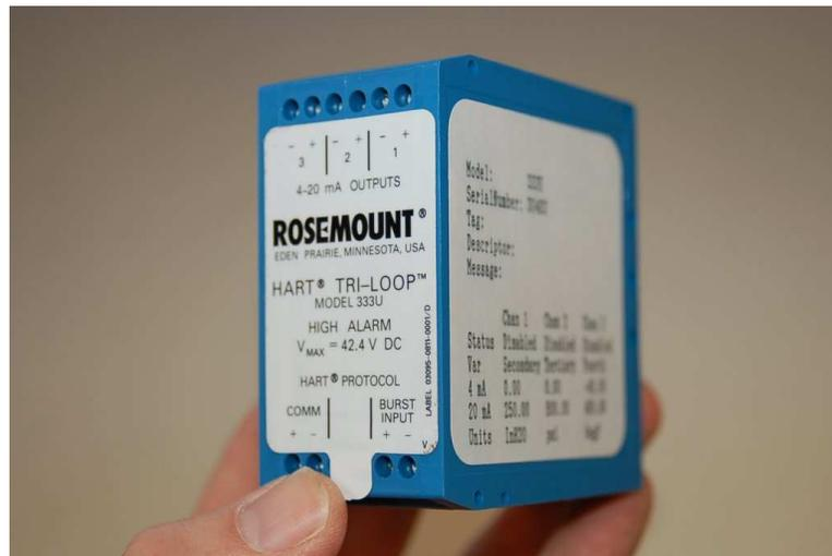
This device polls the multi-variable transmitter and converts up to three HART variables into independent 4-20 mA analog output signals, which any suitable analog indicator or controller device may receive.
