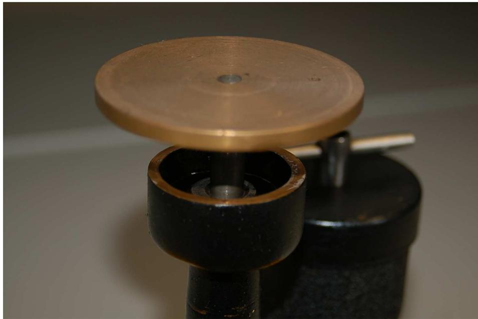
A common operating practice for any deadweight tester is to gently spin the mass during testing so that the primary piston continually rotates within its cylinder. Any motion will prevent static friction from taking hold, helping to ensure the only force on the primary piston is the force of the fluid within the deadweight tester.
