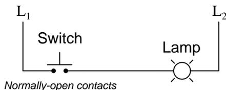
We can tell this switch is a normally-open (NO) switch because it is drawn in an open position. The lamp will energize only if someone presses the switch, holding its normally-open contacts in the “closed” position. Normally-open switch contacts are sometimes referred to in the electrical industry as *form-A* contacts.
