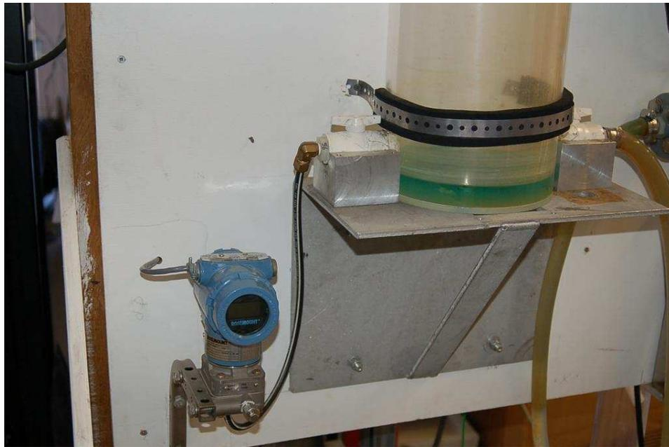
Consider the example of a pressure sensor measuring the level of liquid ethanol in a storage tank. The measurement range for liquid height in this ethanol storage tank is 0 to 40 feet, but the transmitter is located 30 feet below the tank:
