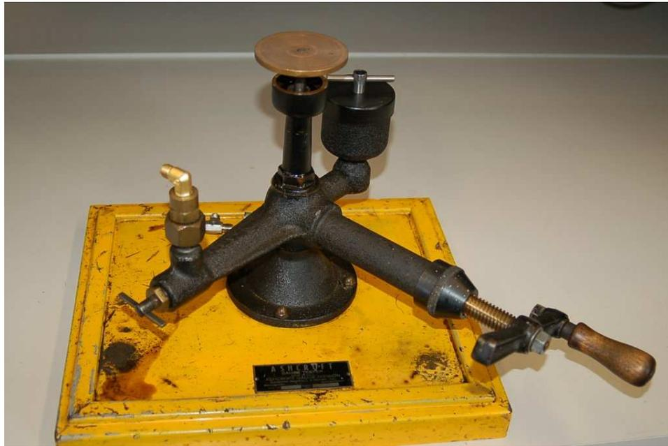
When sufficient pressure has been accumulated inside the tester to overcome the weight on the piston, the piston rises off its rest and “floats” on the pressurized oil, as shown in this close-up photograph:
