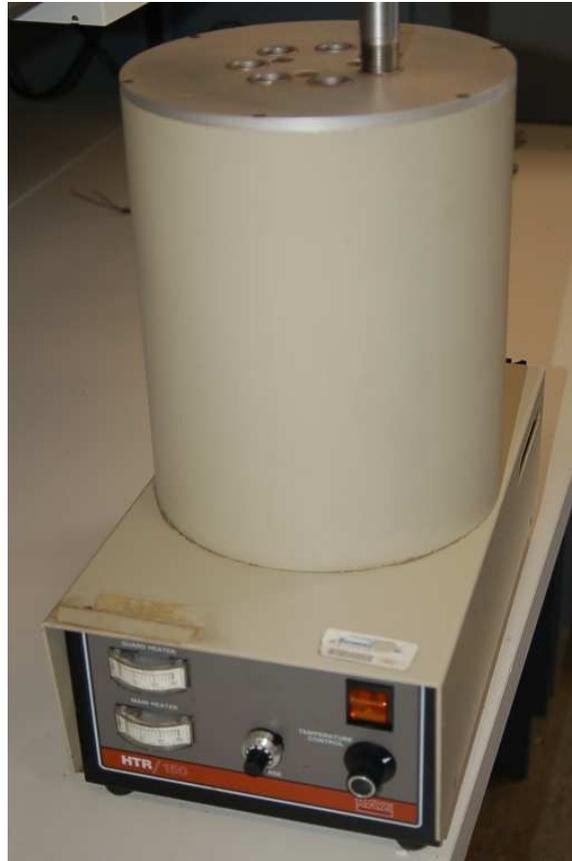
*Dry-block* temperature calibrators also exist for creating accurate calibration temperatures in the instrument shop environment. Instead of a fluid (or fluidized powder) bath as the thermal medium, these devices use metal blocks with blind (dead-end) holes drilled for the insertion of temperature-sensing instruments.
