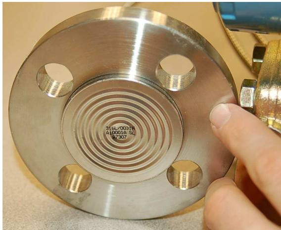
Just like the isolating diaphragms of the pressure-sensing capsule, these remote diaphragms need only transfer process fluid pressure to the fill fluid and (ultimately) to the taut sensing diaphragm inside the instrument. Therefore, these diaphragms perform their function best if they are designed
