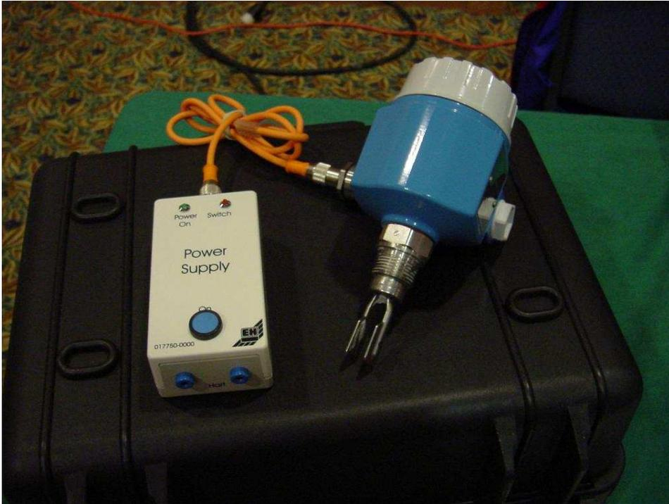
An electronic circuit continuously excites the tuning fork, causing it to mechanically vibrate. When the prongs of the fork contact anything with substantial mass, the resonant frequency of the structure dramatically decreases. The circuit detects this change and indicates the presence of material contacting the fork.
