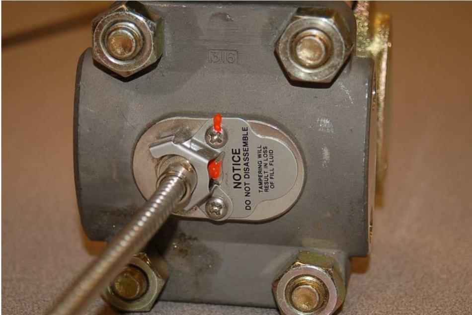
In order for a remote seal system to work, the hydraulic “connection” between the sealing diaphragm and the pressure-sensing element must be completely gas-free so that there will be a “solid” transfer of motion from one end to the other.
