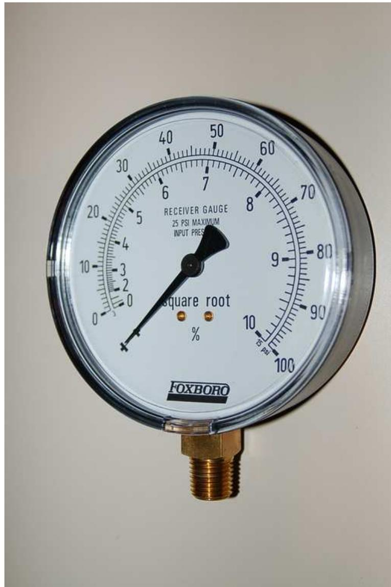
Now, a doubling of fluid flow rate still results in a quadrupling of needle motion, but due to the nonlinear scale this translates into a simple doubling of indicated flow, which is precisely what we need for this to function as an accurate flow indicator.
