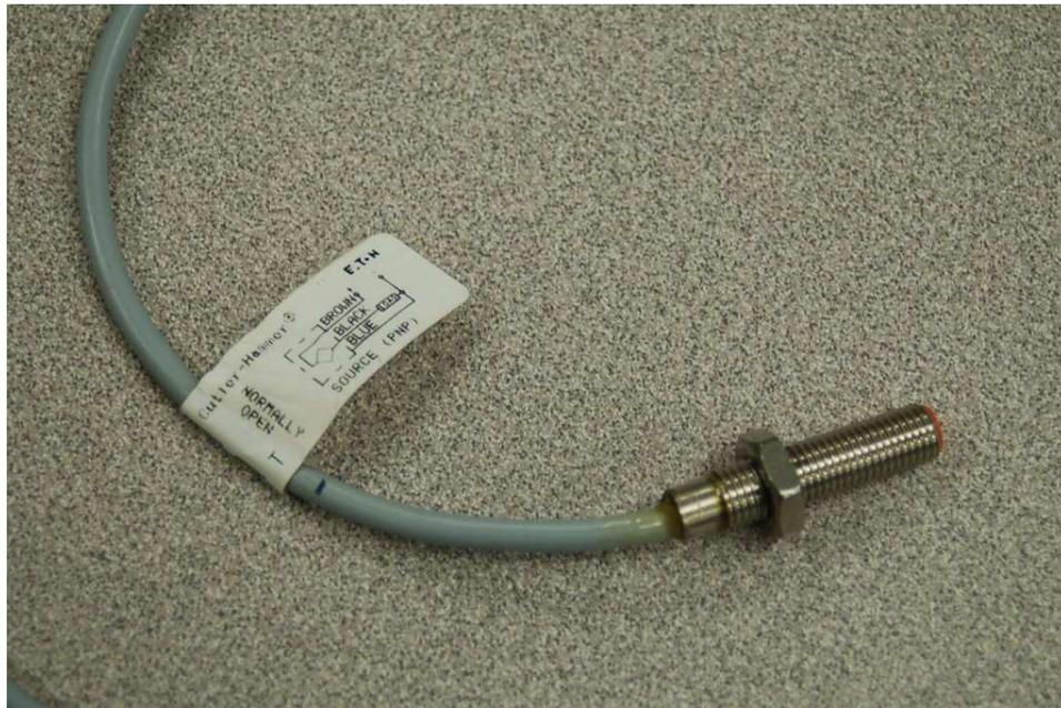
This switch detects the passing of teeth on the chain sprocket, generating a slow square-wave electrical signal as the sprocket rotates. Such a switch may be used as a rotational speed sensor
