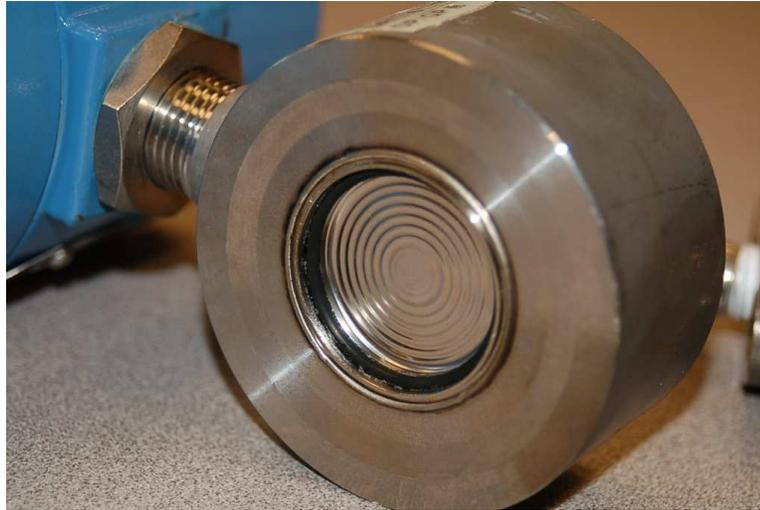
The differential capacitance sensor inherently measures *differences* in pressure applied between its two sides. In keeping with this functionality, this pressure instrument has two threaded ports into which fluid pressure may be applied. A later section in this chapter will elaborate on the utility of differential pressure transmitters (section 12.5 beginning on page 316).
