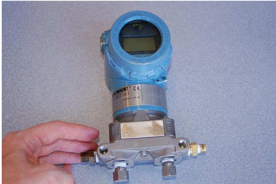
Just like the older model, this instrument has two ports through which fluid pressure may be applied to the sensor. The sensor, in turn, responds only to the *difference* in pressure between the ports.
