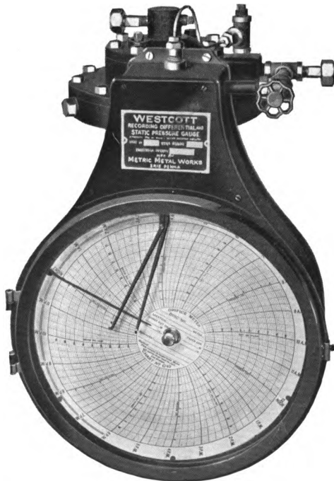
Fig. 53—DIFFERENTIAL GAUGE, 10 INCH DIFFERENTIAL RANGE
