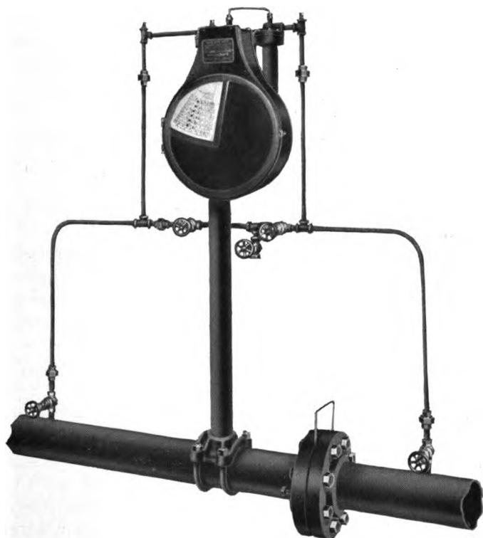
Fig. 58—DIFFERENTIAL GAUGE WHICH INDICATES RATE OF FLOW PER HOUR. IN MEASURING GAS THE RESULT IS READ IN CUBIC FEET PER HOUR. THIS DOES AWAY WITH THE NEED OF PRESSURE EXTENSIONS TO DETERMINE THE RATE OF FLOW. SEE PAGE 299.
