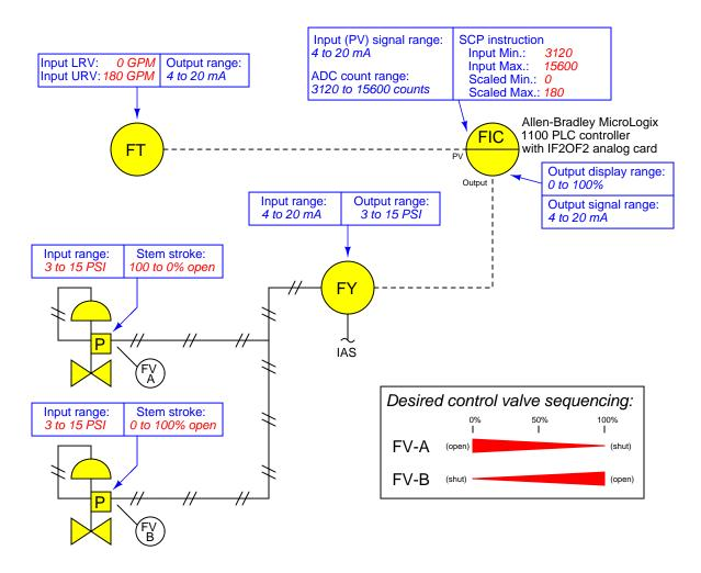
A PV measurement error could lie within the transmitter, or within the controller's analog input. A single current measurement of the transmitter's signal will tell you where the calibration error resides.
