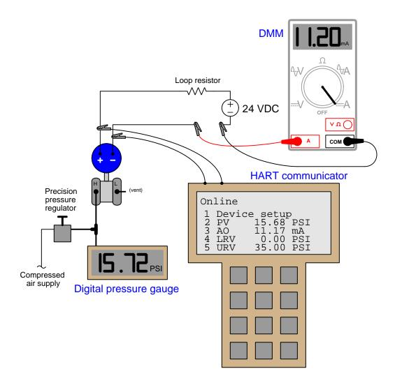
Does this transmitter exhibit a *sensor trim* error, an *output trim* error, or both? If both errors exist, which of the two is more significant?
