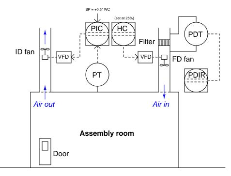
Suppose you are called to troubleshoot a problem in this system: the room air pressure is holding steady at +1.03 inches WC (according to the display on the DDC control system). Based on this data, identify the most likely cause of the problem, and also how you would confirm your diagnosis *before* making any repairs.
