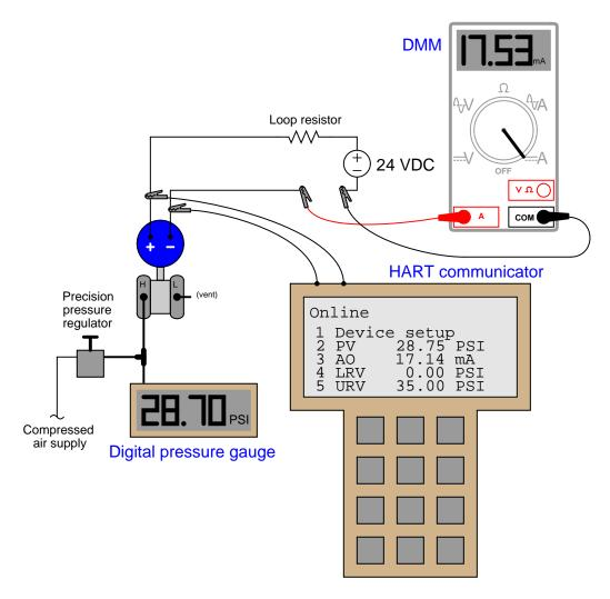
Calculate the amount of *sensor trim* error as well as the amount of *output trim* error, both expressed in percent of span. Also, explain why the HART communicator is necessary to be able to separately calculate these error values.
