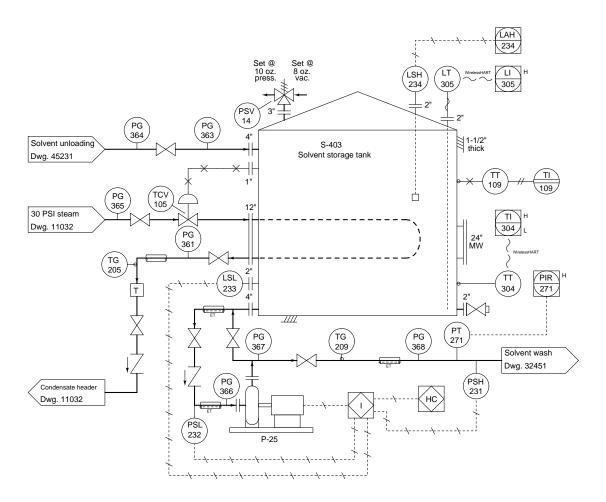
Examine this diagram closely to look for any process vulnerabilities that could be exploited through a cyber-attack (i.e. what adjustments or "spoofing" of variables or changing of modes might be made to the control system after the network has been breached), and what the effects of those attacks might be on the process. Also, identify any instrumentation in this solvent storage tank that appears immune to cyber-attack.
