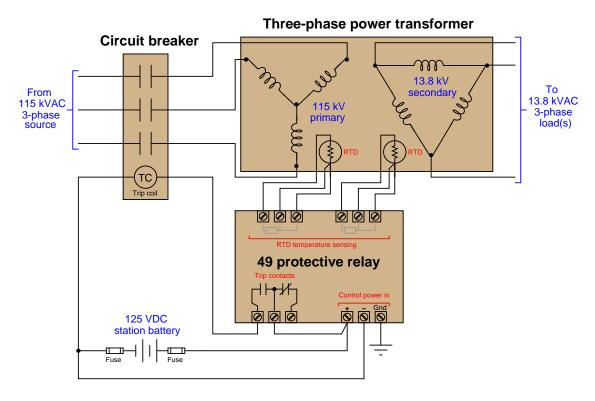
Identify how you would perform an "As-Found" test on this protective relay to ensure it would act to trip the circuit breaker in the event the transformer got too hot, without actually tripping the breaker. In other words, devise a "live" test of the protective relay that does not actually interrupt power to the transformer during the test. Assume the transformer's trip temperature setting is 60 degrees Celsius, and that the formula relating RTD resistance with temperature is as follows:
