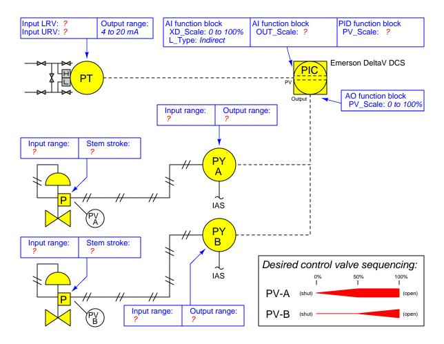
Write the proper range values inside the boxes near each instrument, showing the proper configuration for each instrument needed to achieve the desired result.
