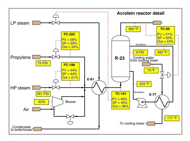
Examine this display closely to look for any process vulnerabilities that could be exploited through a cyber-attack (i.e. what adjustments or "spoofing" of variables or changing of modes might be made to the control system after the network has been breached), and what the effects of those attacks might be on the process.
