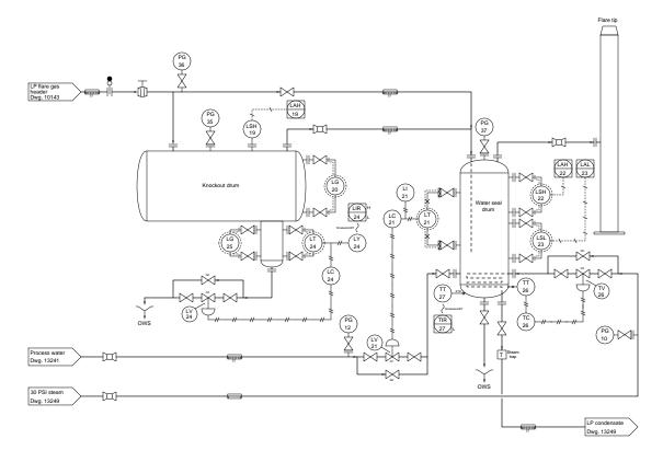
Describe the practical purpose of each controller in this P&ID (i.e. explain the reason why we have a controller installed and working in each case), and then determine its proper action. Assuming all transmitters are direct-acting (greater measured variable = greater signal output), determine the proper action (direct or reverse) for each controller in this system.
