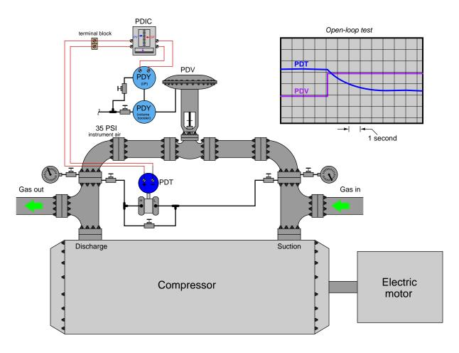
Identify what type of problem you think you are dealing with here, as the compressor's differential pressure should *not* take several seconds to stabilize following a sudden move by the recirculation valve. Also suggest a next diagnostic test or measurement to take, explaining how the result(s) of that test help further identify the location and/or nature of the fault.
