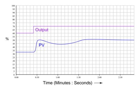
Explain the odd shape of the process variable (PV) trend following the output step-change: why the flow increases, then "sags," then stabilizes. Identify a diagnostic test you could perform on this process to positively identify the source of this strange behavior, explaining how the result(s) of this next test would help you identify the cause.
