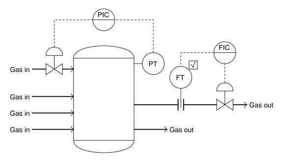
When the flow indicating controller (FIC) is placed in manual mode and the output "bumped" 10%, the result is certainly not what you would expect to see in a liquid flow control system:
