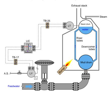
Identify the likelihood of each specified fault for this system. Consider each fault one at a time (i.e. no coincidental faults), determining whether or not each fault could independently account for *all* measurements and symptoms in this system.
