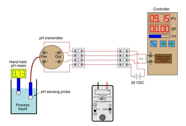
The calibrated range of the 4-wire pH transmitter is supposed to be 2 to 12 pH, with a 4 to 20 mA signal output range. An instrument technician begins to diagnose the problem by taking a loop calibrator and measuring the current signal being sent to the indicating controller. The loop calibrator registers 15.43 milliamps.
