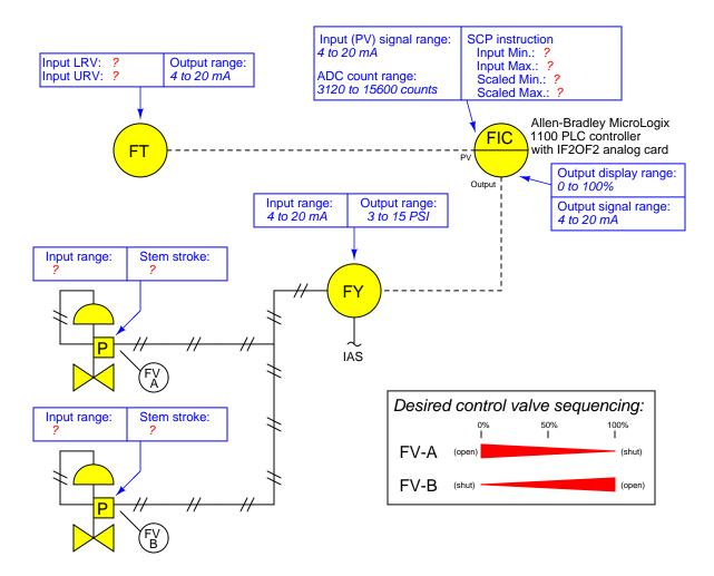
Write the proper range values inside the boxes near each instrument, showing the proper configuration for each instrument needed to achieve the desired result.
