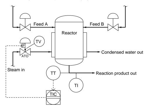
Suppose the last instrument technician to calibrate the temperature transmitter made a mistake, and the transmitter consistently reads  $15^{o}$  too hot. For example, if the reaction product temperature is actually  $275^{o}$  F, the transmitter outputs a current signal corresponding to  $290^{o}$  F.
