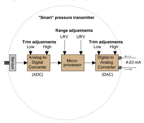
The purpose of the analog-to-digital converter (ADC) is to translate the pressure sensor's electrical output signal into a digital number the microprocessor can understand. Likewise, the purpose of the digital-to-analog converter (DAC) is to translate the digital output of the microprocessor into a 4 to 20 mA DC current signal representing measured pressure. The procedure of calibrating the ADC is called a *sensor trim*, while the process of calibrating the DAC is called an *output trim*.
