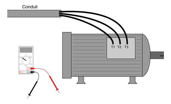
List all possible pairs of points the electrician must check for voltage between. Don't forget to include earth ground as one of those points, in addition to T1, T2, and T3!
