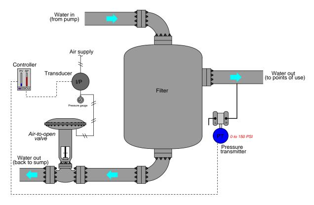
Your first test is to measure loop current in the circuit connecting the pressure transmitter to the pressure controller. There, your multimeter registers 6.88 milliamps. Your next step is to record the pressure gauge's indication (at the I/P output tube): 7.5 PSI.
