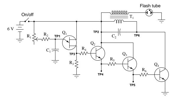
Turning the flash rate control (rheostat  $R_1$ ) to the slowest position, you take two voltage measurements with a voltmeter: at test point 3 (between TP3 and ground) you measure a voltage rhythmically pulsating between about 1.5 and 4 volts DC. At test point 6 (between TP6 and ground) you measure about 0.3 volts DC all the time.
