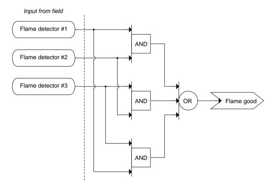
The purpose of this logic system is to indicate whether or not at least *two* flame detectors are showing the presence of flame in a burner system. Here, flame is good, and no flame is bad. Explain how this logic system works, and relate the symbols contained within to traditional logic symbols such as these shown below:
