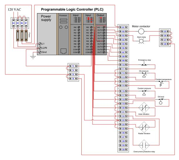
Noting the status of the LEDs on the discrete input card of the PLC while the compressor is running as it should, identify what you would have to do to electrically simulate the following trip conditions (i.e. make the PLC "think" that a dangerous condition existed when in fact one did not):
