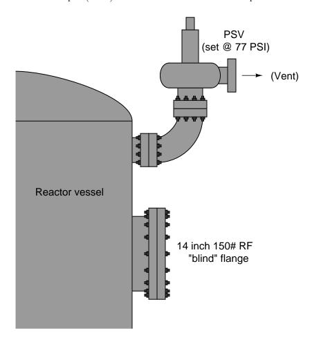
Calculate the total force exerted on a 14 inch blind flange located on the side of the reactor at the PSV lift pressure, both in pounds and in tons. Use  $13\frac{1}{4}$  inches as the effective diameter of the blind flange.
