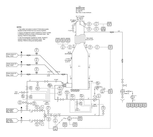
Fuel pressure safety switches on a BMS are typically wired for *de-energize to trip* operation. Given this design specification, determine whether the following pressure switches should be wired as *normally-open* (NO) or *normally-closed* (NC), assuming we have the option of choosing for each switch:
