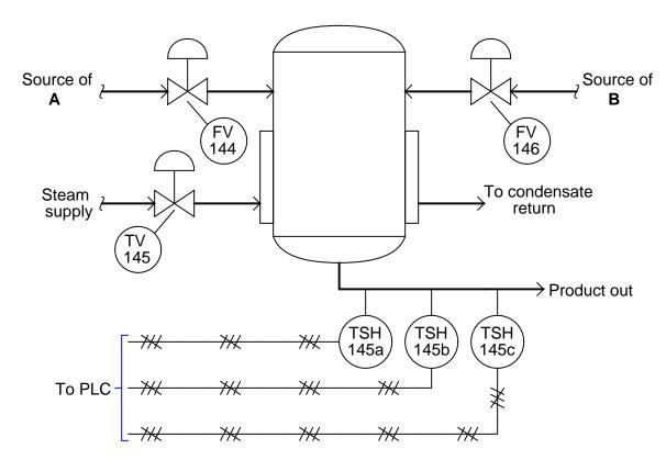
Three temperature switches connect to a PLC, triggering an automatic shutdown of the process if at least two of the three switches register too-cold temperatures (2003 shutdown).
