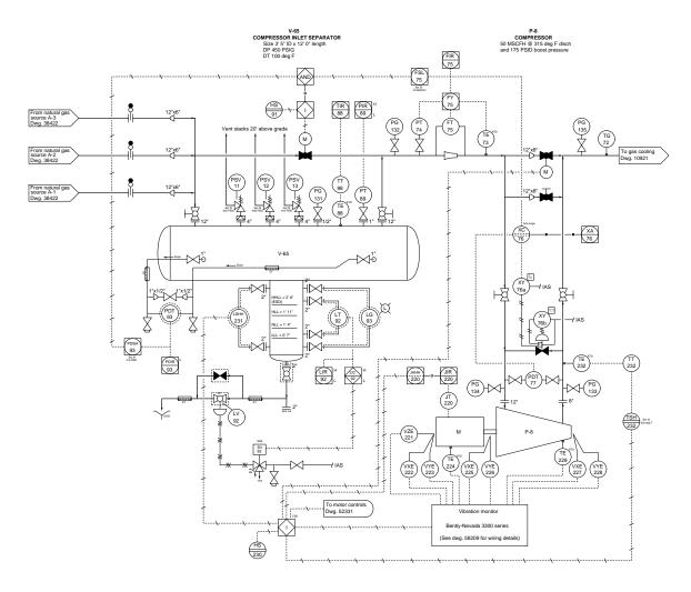
Examine this diagram closely to look for any potential vulnerabilities in the instrumentation that could be exploited through a cyber-attack, and what the effects of those attacks might be on the process. Also, identify any instrumentation in this compressor system that appears immune to cyber-attack.
