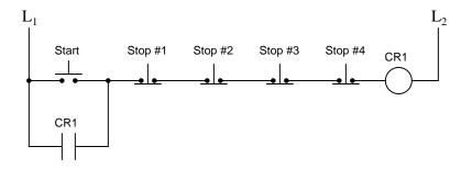
Determine the *dependability* of this safety shutdown system in terms of how many "Stop" switches would have to be actuated to halt the conveyor. Conversely, determine the *security* of this system in terms of how many "Stop" switches must be returned to their proper (running) positions in order to start the conveyor up.
