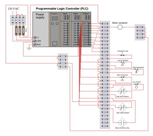
Identify the "trip state" for each of the PLC inputs (sensing switches): whether each input must *energize* or *de-energize* to trip the compressor. Note that the PLC input channels are not drawn here showing operating conditions (i.e. there are no LED lights shown in an illuminated state to help you determine switch status).
