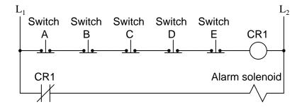
Write the Boolean expression for this relay circuit, then simplify that expression using DeMorgan's Theorem and draw a new relay circuit implementing the simplified expression.
