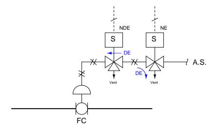
Identify the "normal" mode of operation for this system as specified by the process engineer who built it: the status of the process valve and of both solenoid valves during typical process operations.
