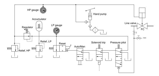
Identify all spool valve positions, and also trace the direction of oil flow, following a solenoid "trip" event.
