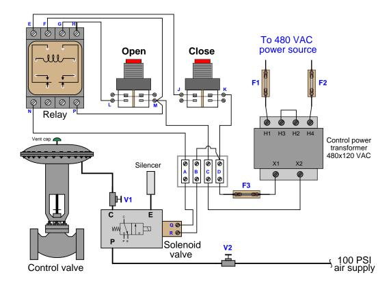
You measure 0 volts AC between terminals  $\mathbf{C}$  and  $\mathbf{D}$  on the terminal strip, and then switching your multimeter to "resistance" you read a few ohms of resistance between the same two terminals.
