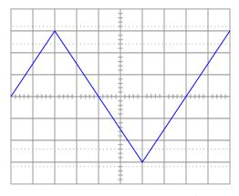
Vertical sensitivity = 10 volts/div 1:1 probe DC coupling Timebase =  $5 \mu s/div$
