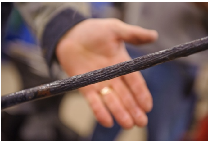
Branch forged under the power hammer using texturing dies
