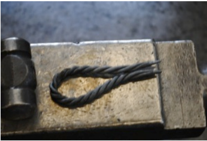
Twist for Poker Handle Ready to Forge Weld
