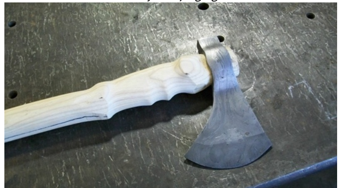
Avery's Damascus hawk forged from double row #60 roller chain with the new handle that he has been making
