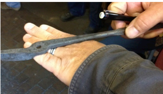
Turn Left on Far Edge to Form the Front of Bolster
