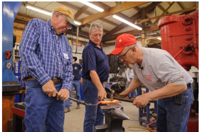
Using a chisel to add tail feathers; Roy Bloom (left) and David Farley (center) assist
