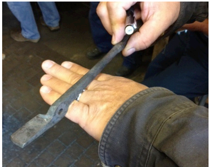
Turn Left on Far Edge to Shape the Back of Bolster
