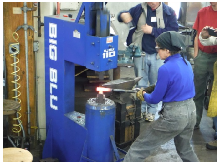
Roberta Demonstrates Pipe Forging on the Power Hammer
