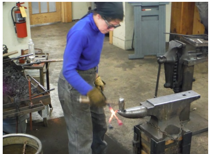
Shaping the Candelabra on the Horn
