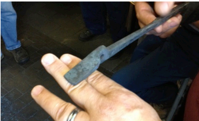
The Progression - Forge the Blade on Near Edge
